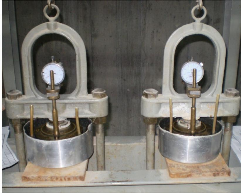
Figure 5.18 View from Oedometers during testing
