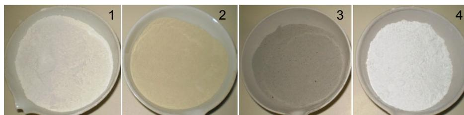
Figure 5.1. Views from Materials (1-kaolinite, 2-bentonite, 3-fly ash, 4-lime)
