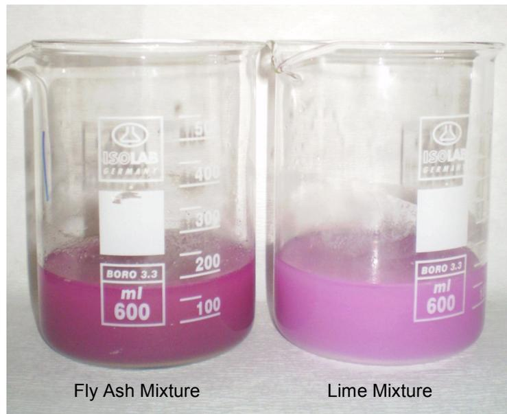
Figure 5.2.View from mixtures before titration
