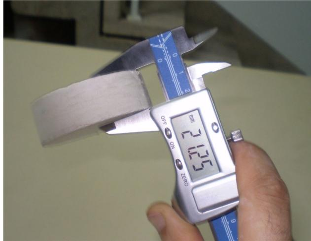
Figure 5.19 Measuring height with digital caliper
