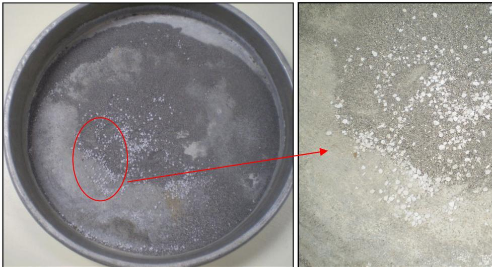
Figure 5.4. Crystals formed in fly ash during the hydrometer test
