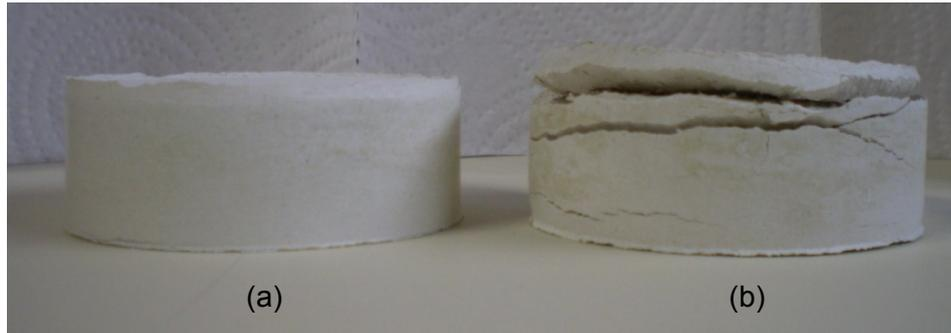
Figure 6.1. Views From 3% lime treated sample after drying ((a)-before first cycle, (b) – before second cycle)
