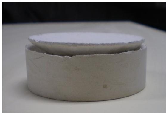
Figure 6.2. View from fungi-shaped heaves occurred in the upper portion of 5% lime treated sample
