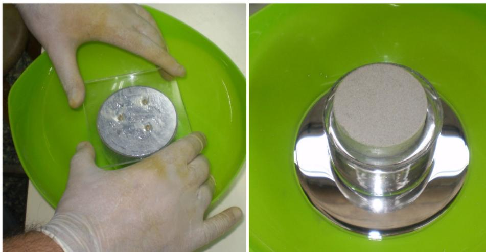
Figure 5.20 Measuring volume with mercury
