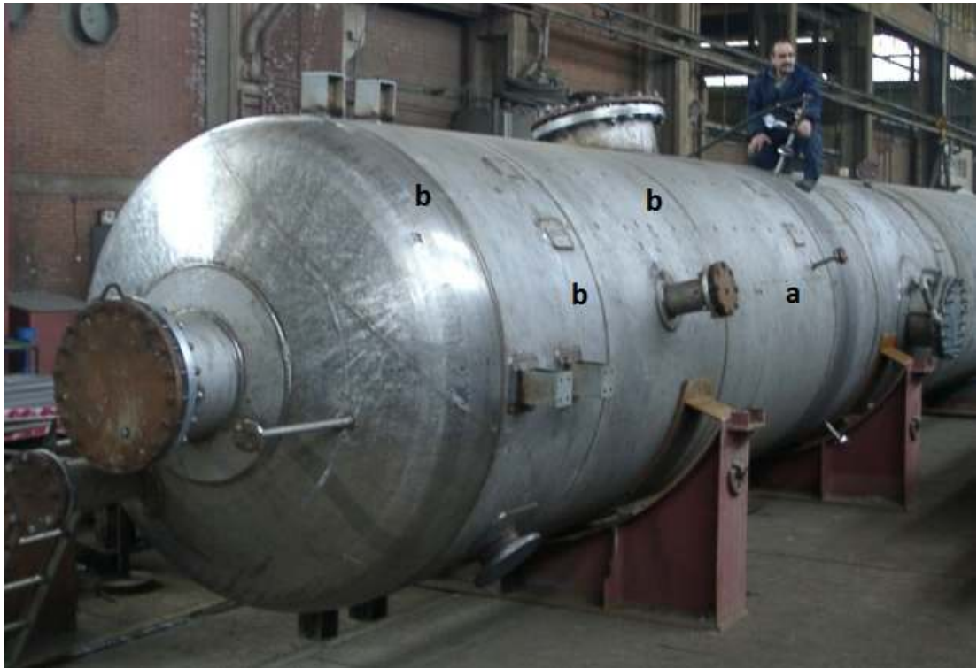
Figure 8: A typical pressure vessel while being manufactured; (a) longitudinal and (b) circumferential joints (GAMA Industrial Plants Manufacturing and Erection, Inc.).
