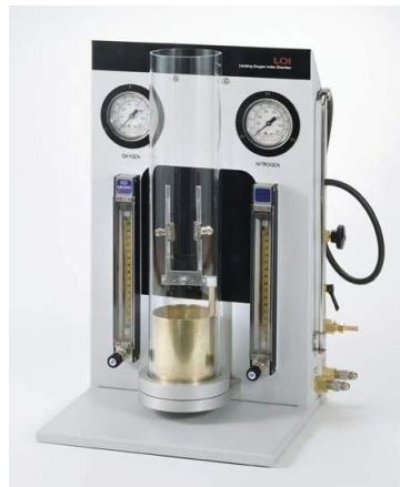
Figure 3.10 Picture of Limiting Oxygen Index test instrument
