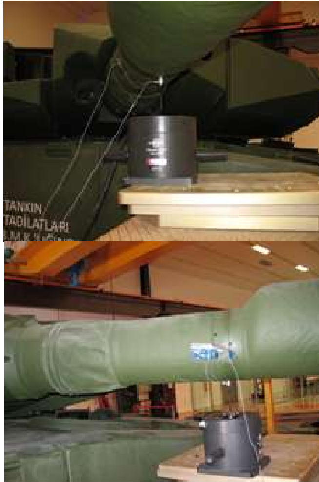
Figure 4-29 Shaker is located around the second accelerometer.
