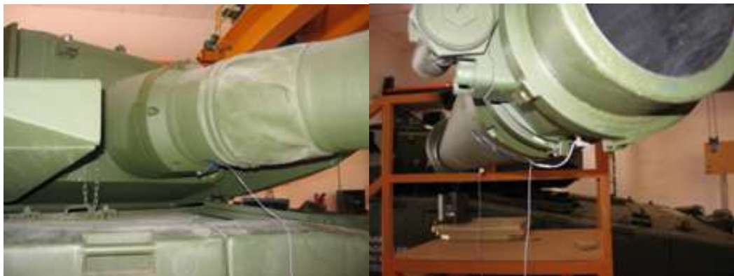
Figure 4-28 Accelerometers are fixed to the gun barrel on several positions.
