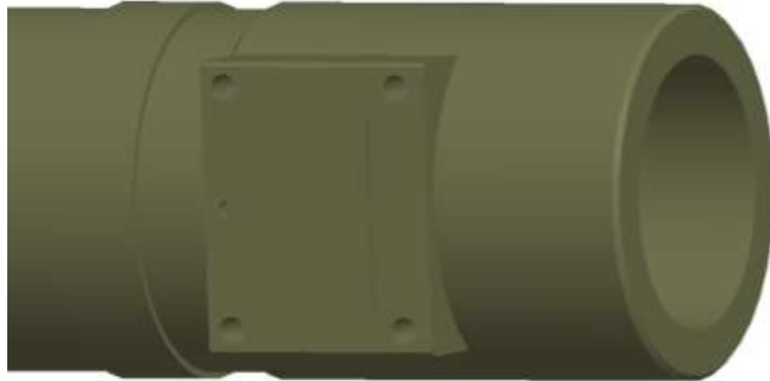
Figure 5-25. Barrel free end with MRS mechanical interface.
