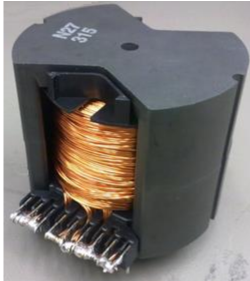
Figure 4-14 Designed and implemented coupled-inductor, photograph 1
