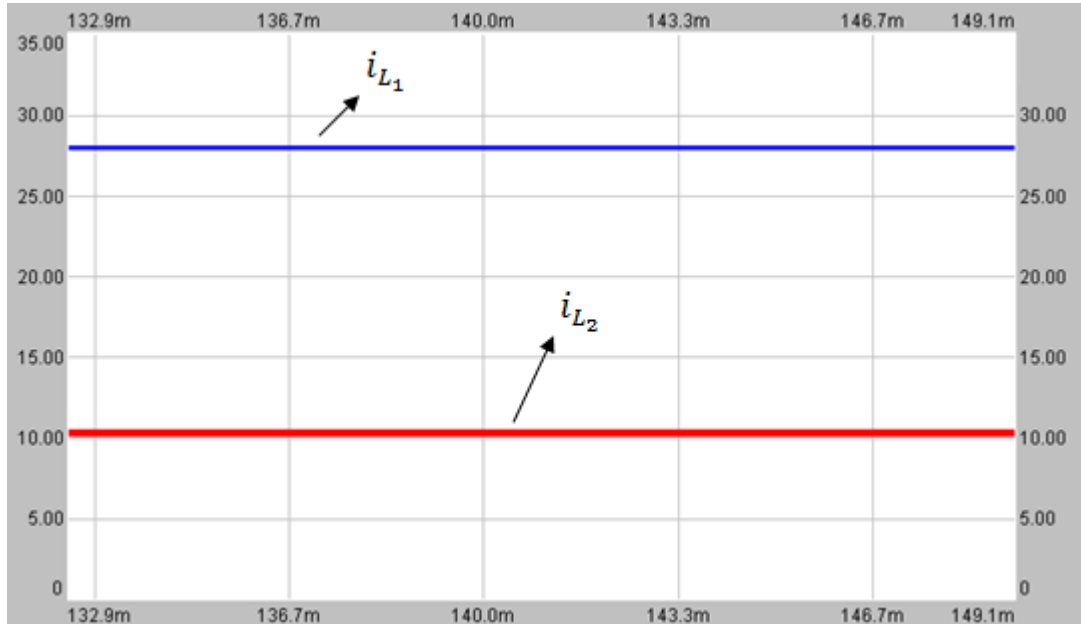
Figure 2-20 i_{L_1} and i_{L_2} waveforms in ripple-free input current case with parasitic elements at full load
