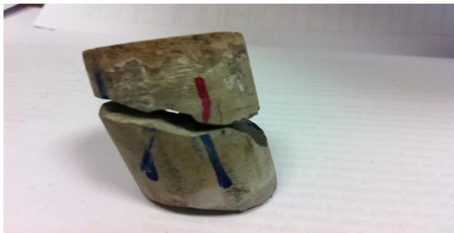
**Fig H.2 Photograph of cement plug # 1 after experiment**
