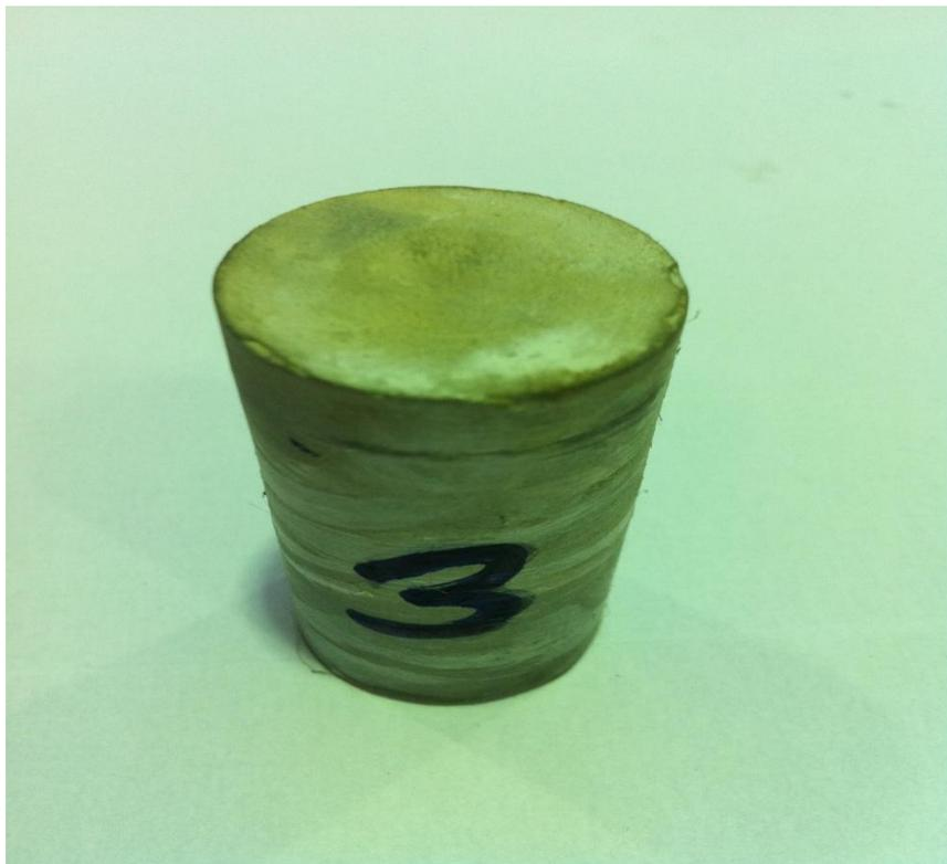
**Fig H.4 Photograph of cement plug# 3 after experiment**
