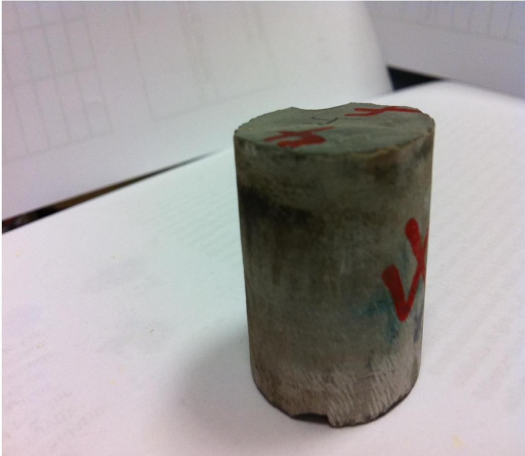
**Fig H.5 Photograph of cement plug # 4 after experiment**
