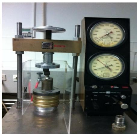
**Fig G.1 Schematic of Versa-Tester Apparatus**
