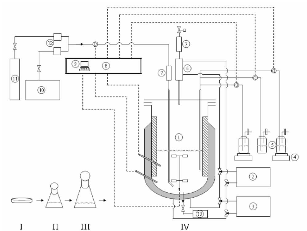
**Figure 3.2** Scheme of the Biostat CT2-2 fermenter system (1) Bioreaction vessel, Biostat CT2-2 (2) Cooling circulator (3) Steam generator (4) Balances (5) Feed, base and antifoam bottles (6) Exhaust cooler (7) Gas filters (8) Controller (9) Biostat CT Software (10) Air compressor (11) Pure O<sub>2</sub> tank (12) Digital mass flow controllers (13) Sample valve (Çelik, 2008)
