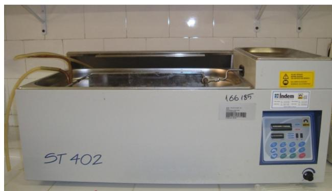
**Figure 4.1** ST 402 Shaking Water Bath
