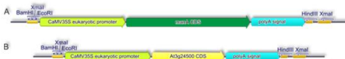
Figure 3.41: Flanking restriction sites of 35S-ManA/MBF1c-NOS cassettes Restriction sites designed for sub cloning of CaMV35SS-ManA-TNOS (A) and CaMV35SS-MBF1c-TNOS (B) cassettes. Note the spatial organization of the restriction sites. The BamHI and EcoRI restriction sites at 5' end of the cassettes are overlapping with an XmaI restriction site in between. That is the three restriction sites each with six bps recognition sequence are stacked into 15 bps length. On the other hand the two restriction sites at 3' end of the cassettes are not overlapping.
