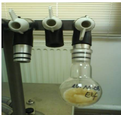
Figure 2.2 Lyophilization of Plant material in Heto, lyophilizator.
