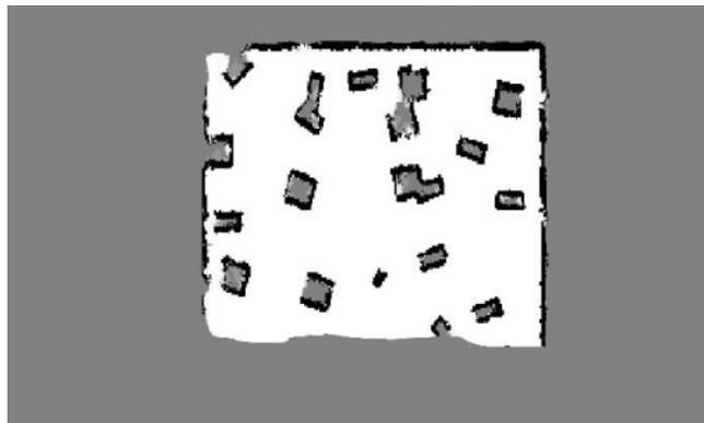
Figure 5.12: Partial occupancy grid environment map of first robot after search and rescue operation.
