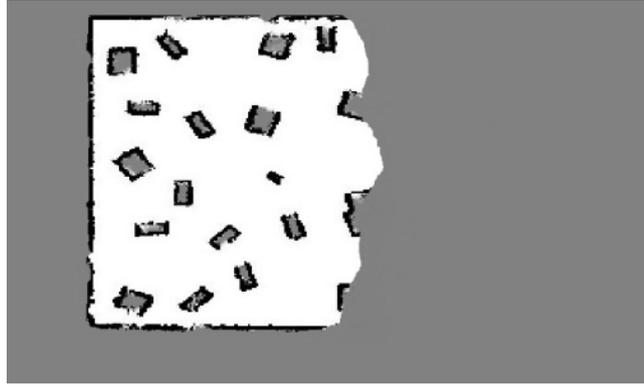
Figure 5.11: Partial occupancy grid environment map of first robot after search and rescue operation.
