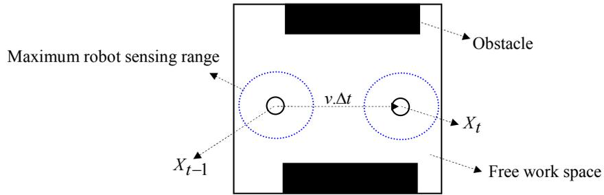
Figure 4.12: Movement representation of the search and rescue robot between  $X_{t-1}$  and  $X_t$  positions.
