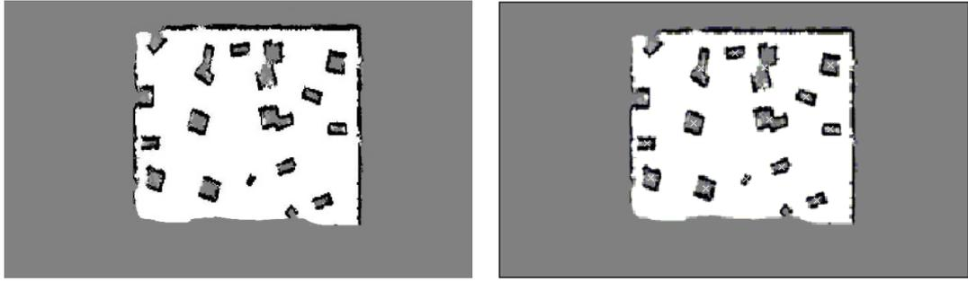
Figure 5.16: Connected component (obstacle) labeling for second robot map, using binary map.
