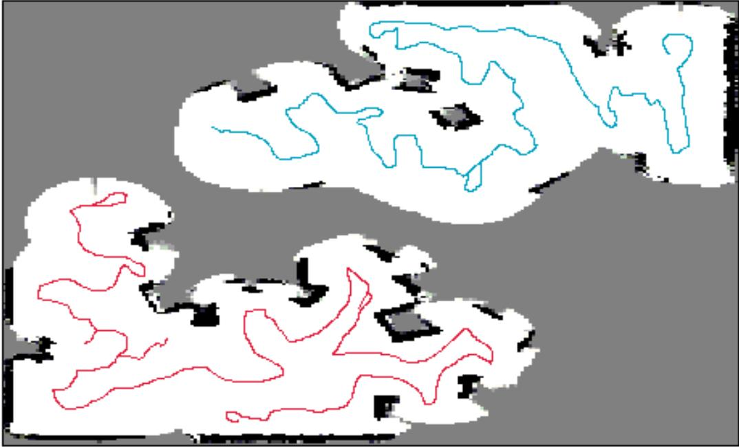
Figure 5.8: Generated environment occupancy grid map of the work space and navigation path of each robot, red colored for first robot and blue colored for other robot unit.
