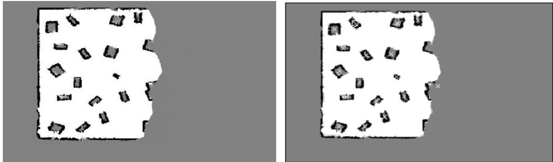
Figure 5.15: Connected component (obstacle) labeling for first robot map, using binary map.
