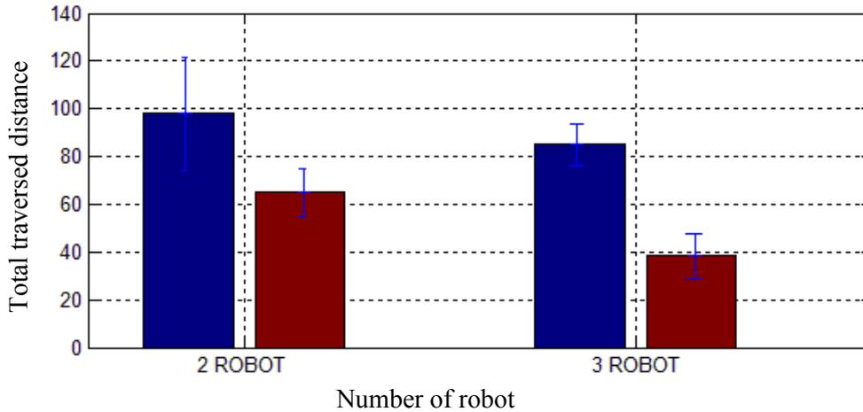
Figure 5.21: Average exploration distances with different number of robots.
