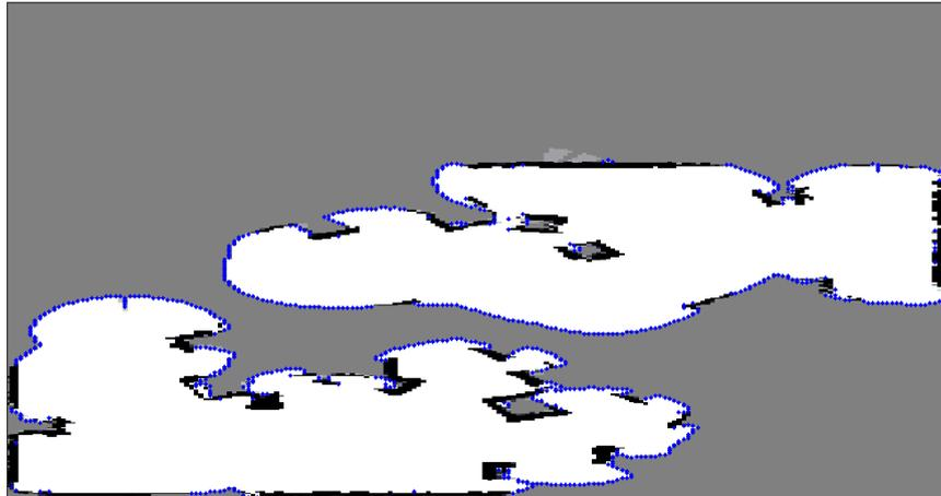
Figure 4.9: Occupancy grid environment map and frontier cell locations (Blue cells) at a specific time  $t$ .
