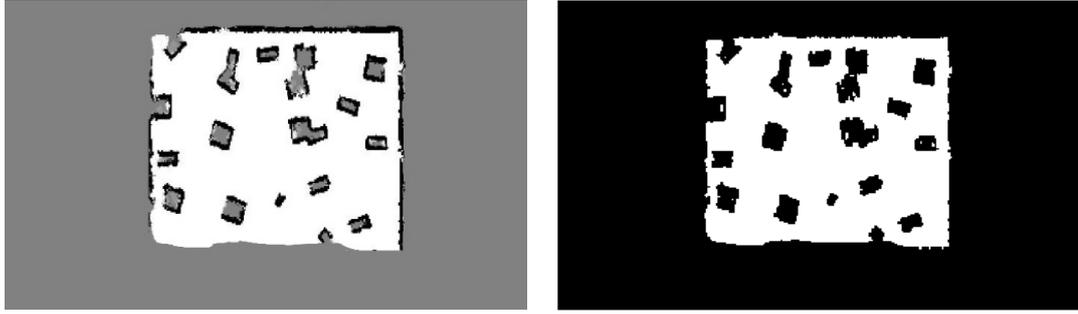
Figure 5.14: Occupancy grid map of second robot and binary representation of it, respectively.
