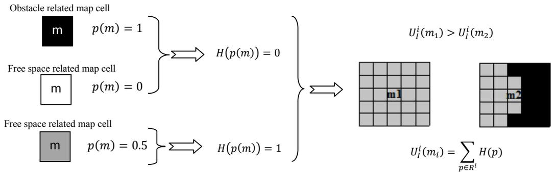
Figure 4.10: Visual example about expected information gain and entropy around an occupancy grid cell  $m$ .
