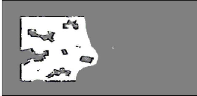
Figure 4.21: Connected component determination and labeling.
