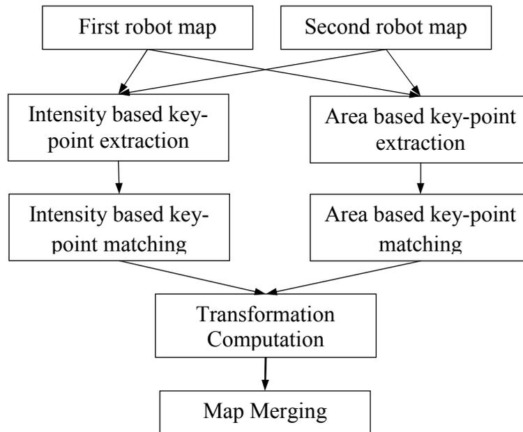
Figure 4.13: Flow chart of proposed occupancy grid map merging algorithm.
