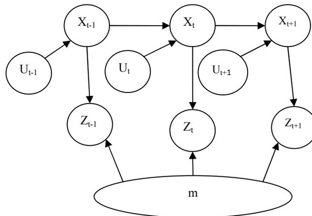
Figure 3.2: Graphical representation of the Simultaneous Localization and Mapping problem [38].
