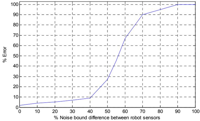
Figure 5.23: Map merging error according to the noise bound difference between robots.
