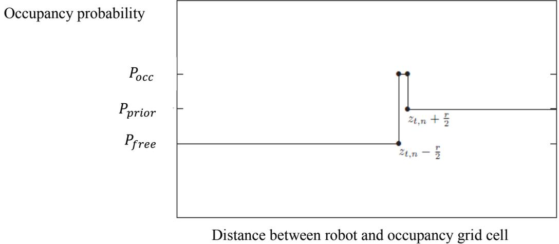
Figure 3.4: Laser sensor model of robot units.
