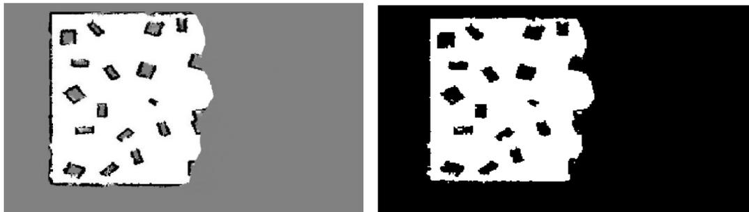
Figure 5.13: Occupancy grid map of first robot and binary representation of it, respectively.
