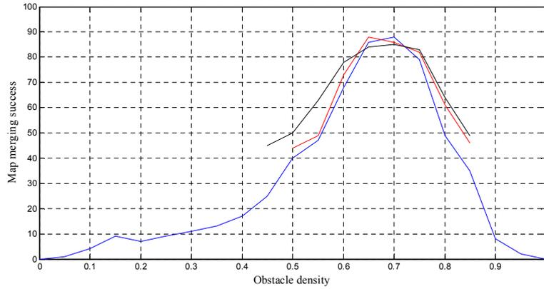
Figure 5.20: Map merging performance according to the environment complexity for different environments.
