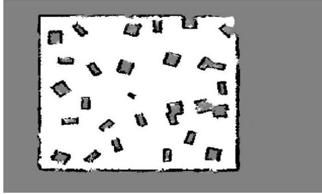
Figure 5.18: Joint and global occupancy grid map of search and rescue environment after the map merging operation.
