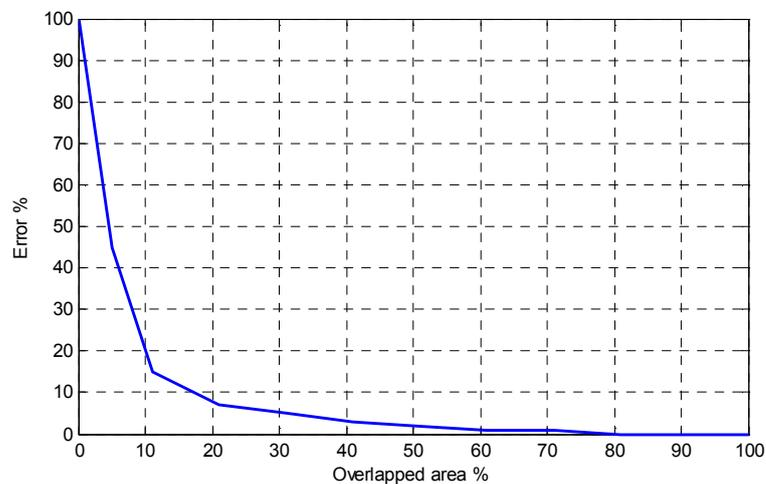
Figure 5.22: Map merging error according to the overlapped area between occupancy grid robot maps.
