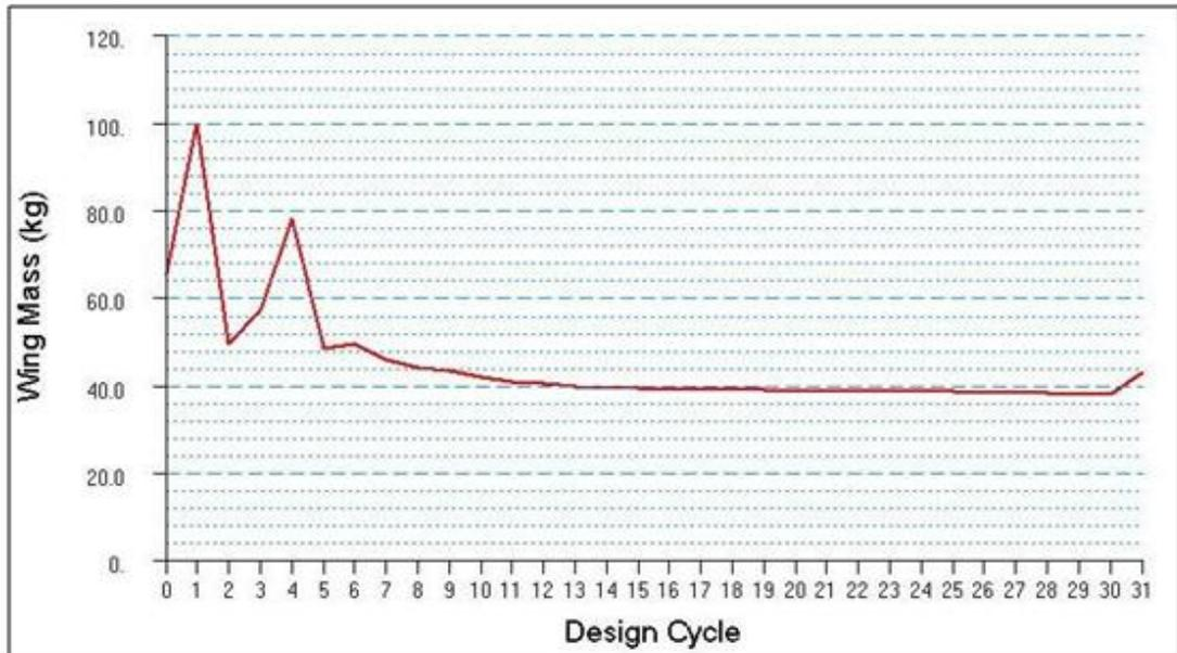
**Figure 4.37:** Variation of the Mass of Wing with Respect to the Design Cycle - Coarse Mesh Beam/Membrane-R Model
