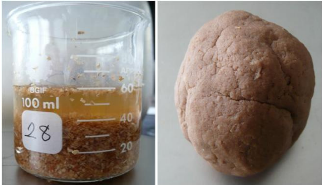
Figure 3. 1 Wheat bran (on the left) and Wheat bran fiber (on the right) containing 90% water
