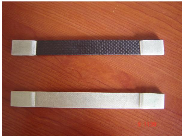
Figure C2: *Specimens after tabs are glued*
