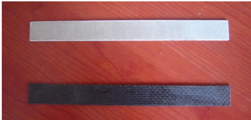
Figure C1: *Specimens prepared according to ASTM D 3039/D 3039M*
