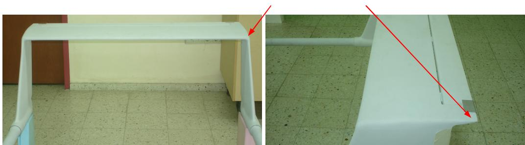
Figure 28: Permanent connection of the horizontal and vertical tail
