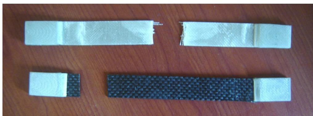
Figure C3: Specimens after the tensile tests
