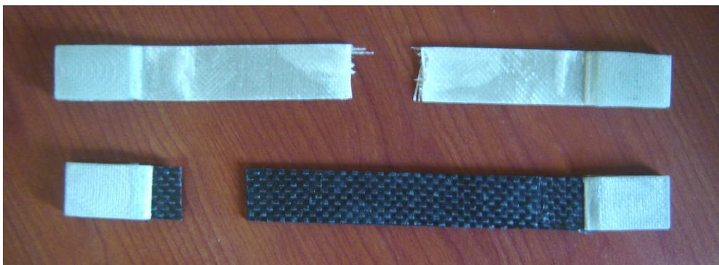
Figure C3: Specimens after the tensile tests
