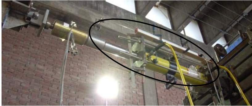
Figure 62: LVDT of 500 mm to measure the lateral top displacement and hydraulic piston
