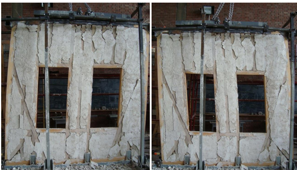
Figure 113: Frame#4 with brick infill after the test
