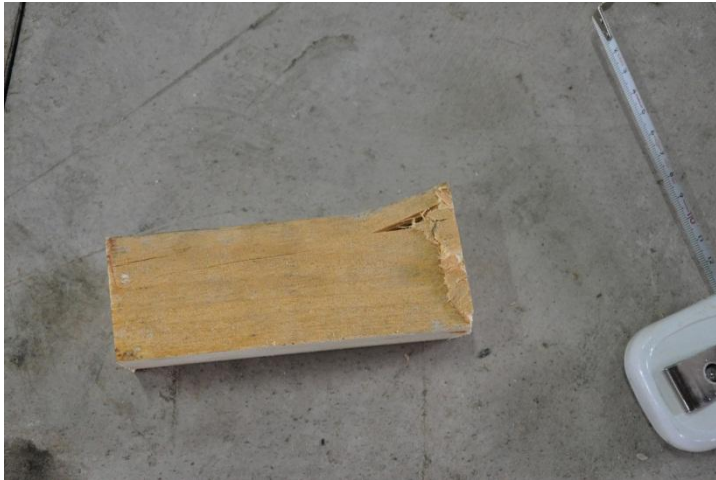
Figure 202: A distorted specimen (yellow pine #1) after compression test parallel to grains
