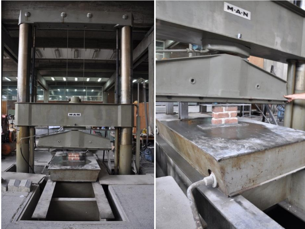
Figure 182: The equipment where compression tests were achieved
