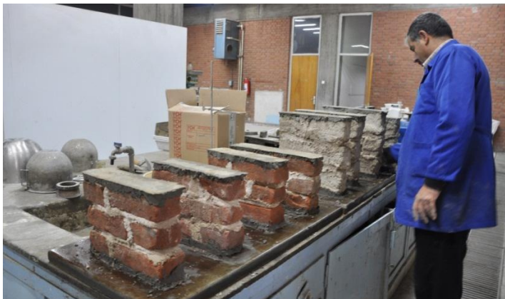
Figure 181: Adobe and brick masonry samples after capping
