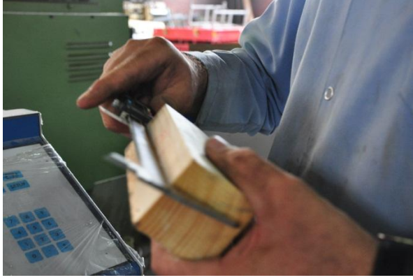
Figure 201: Measurement of the specimen lengths
