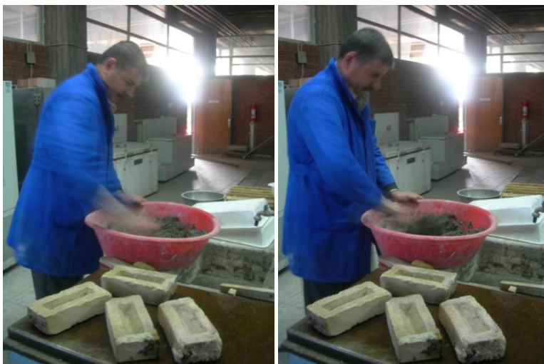
Figure 177: Cement based mortar was prepared for capping
