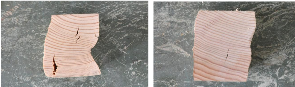
Figure 206: Distorted shapes of two 50x50x95 specimens, loaded beyond their ultimate strengths
