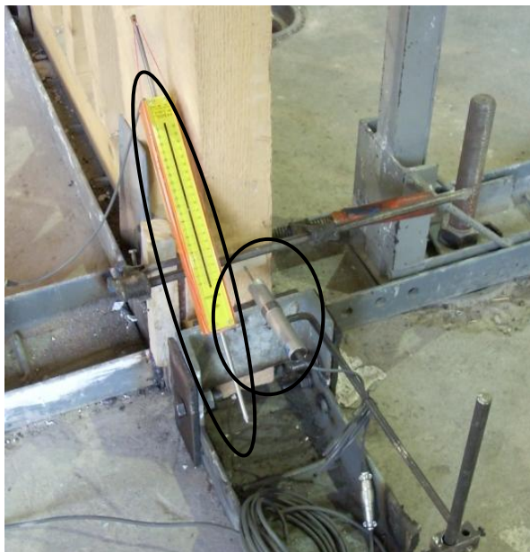
Figure 61: LVDT of 200 mm to measure diagonal displacement and that of 50 mm to check bottom lateral displacement
