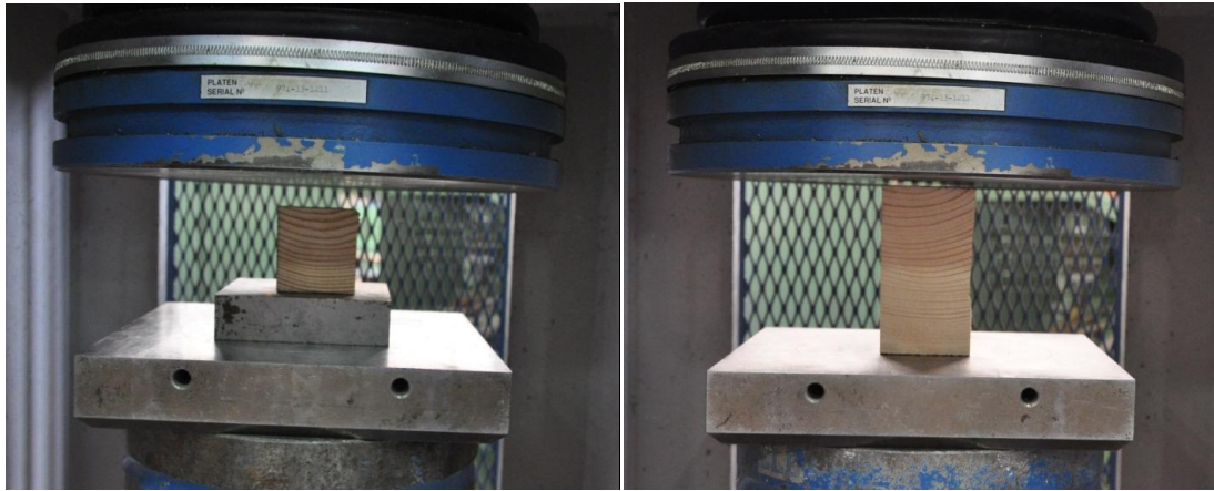
Figure 203: Compression test perpendicular to grains
