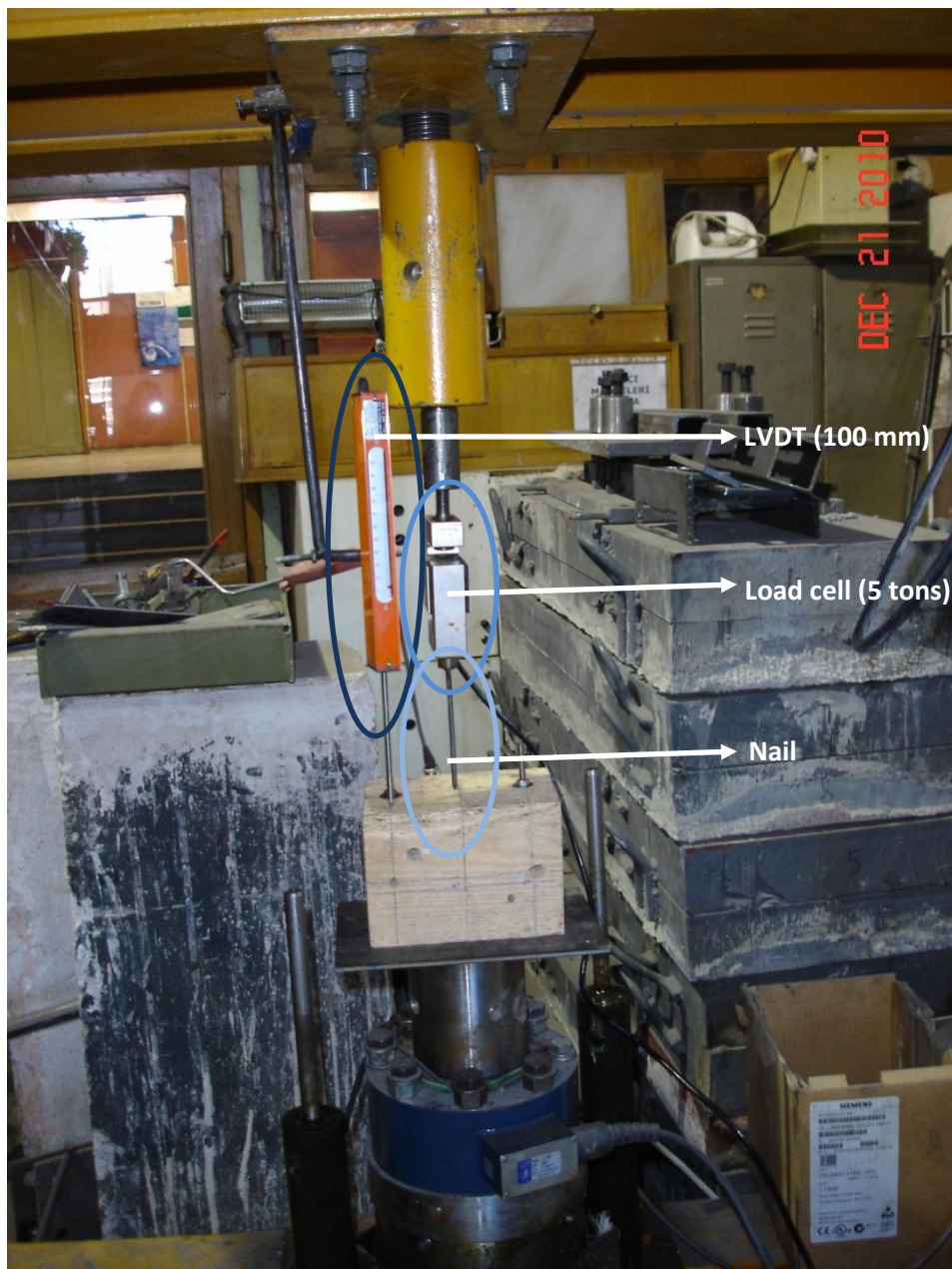
Figure 188: Test set-up used for pull-in/out tests
