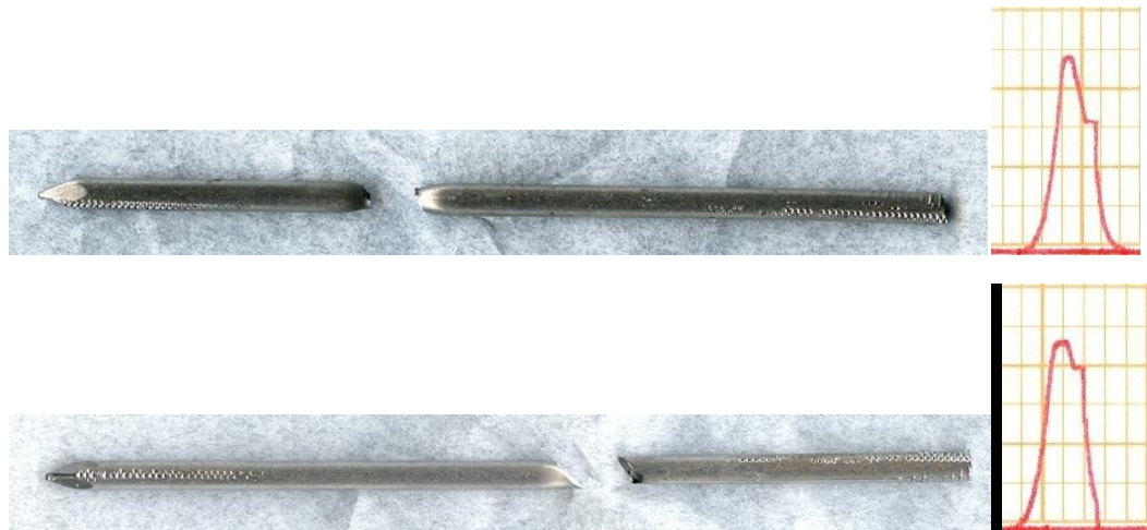
Figure 184: Nails after tension test
