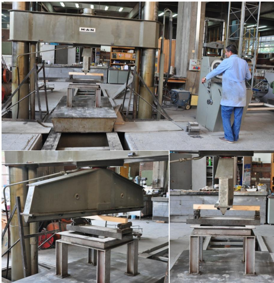
Figure 194: Overall view of the instrument, where bending tests were carried out
