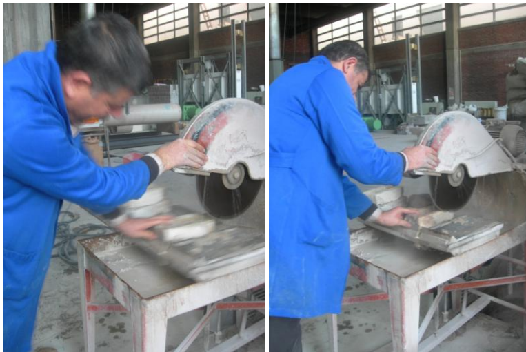
Figure 176: Before capping the adobe and brick samples, their edges were adjusted by cutting
