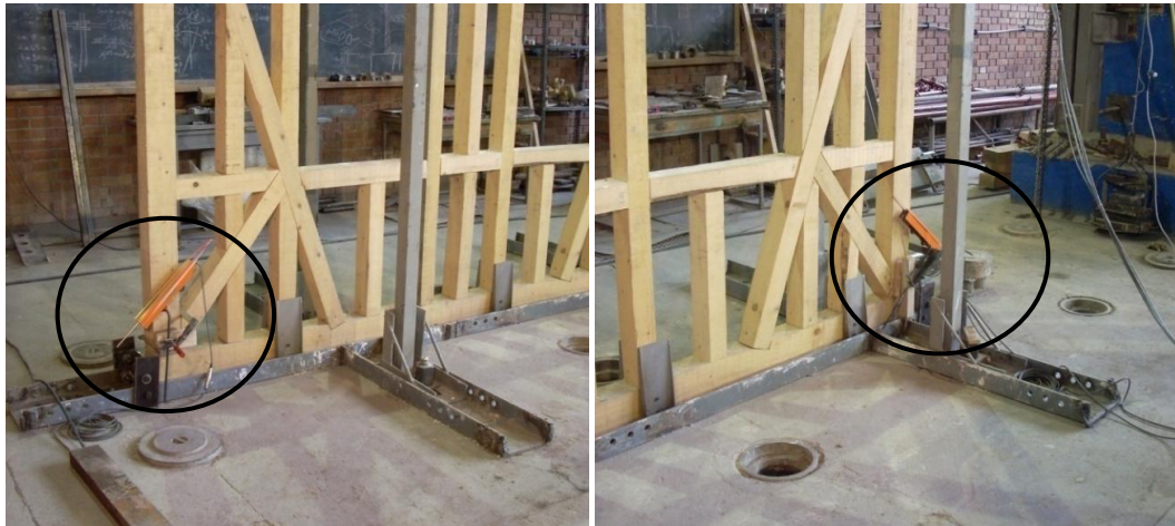
Figure 60: LVDTs of 200 mm placed at both sides of the frame to measure diagonal displacement
