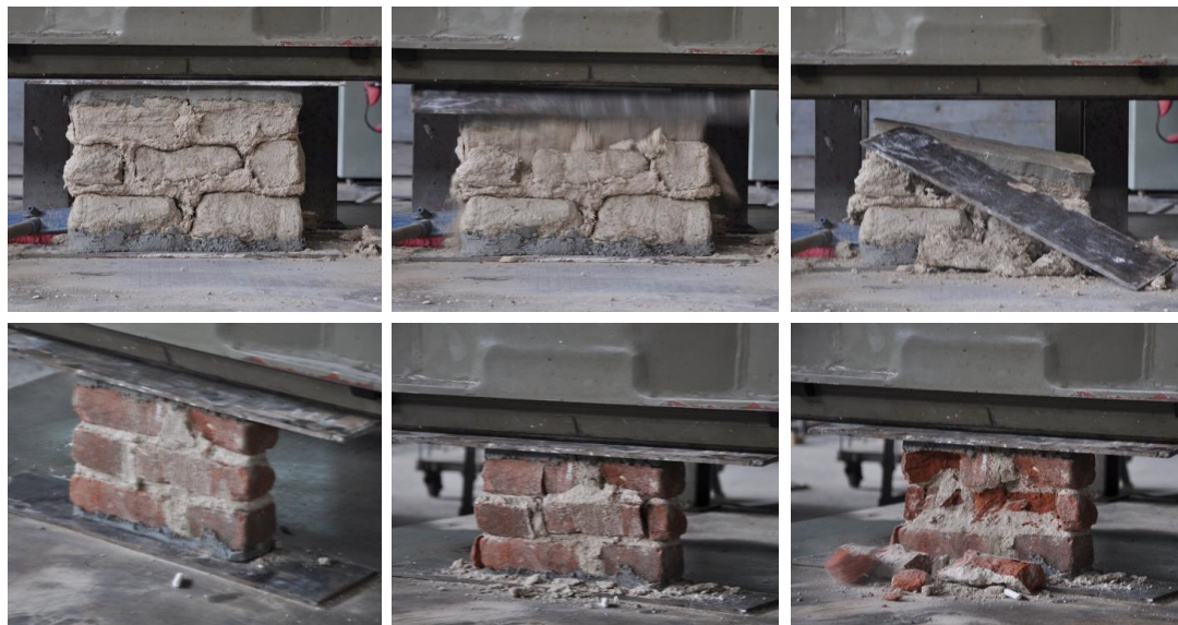
Figure 183: Two examples to the failures of adobe and brick masonry samples under compression
