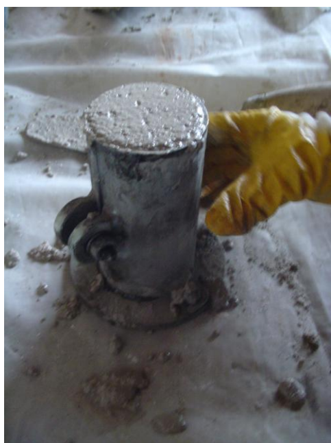
Figure 175: Plaster and mortar samples taken by standard sampling cylinders
