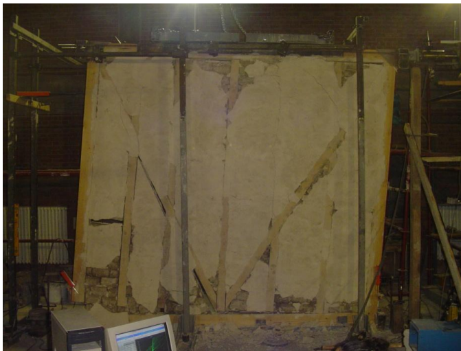
Figure 87: Frame#2 with adobe infill after test
