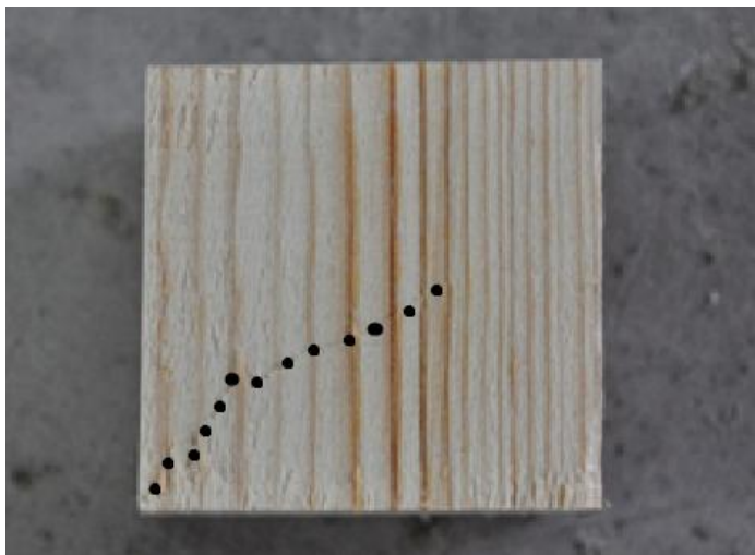
Figure 207: A cracked specimen after compression test parallel to grains
