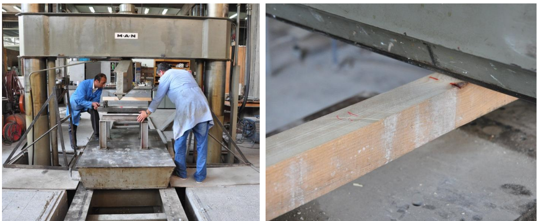
Figure 196: Adjusting the specimen for a central loading
