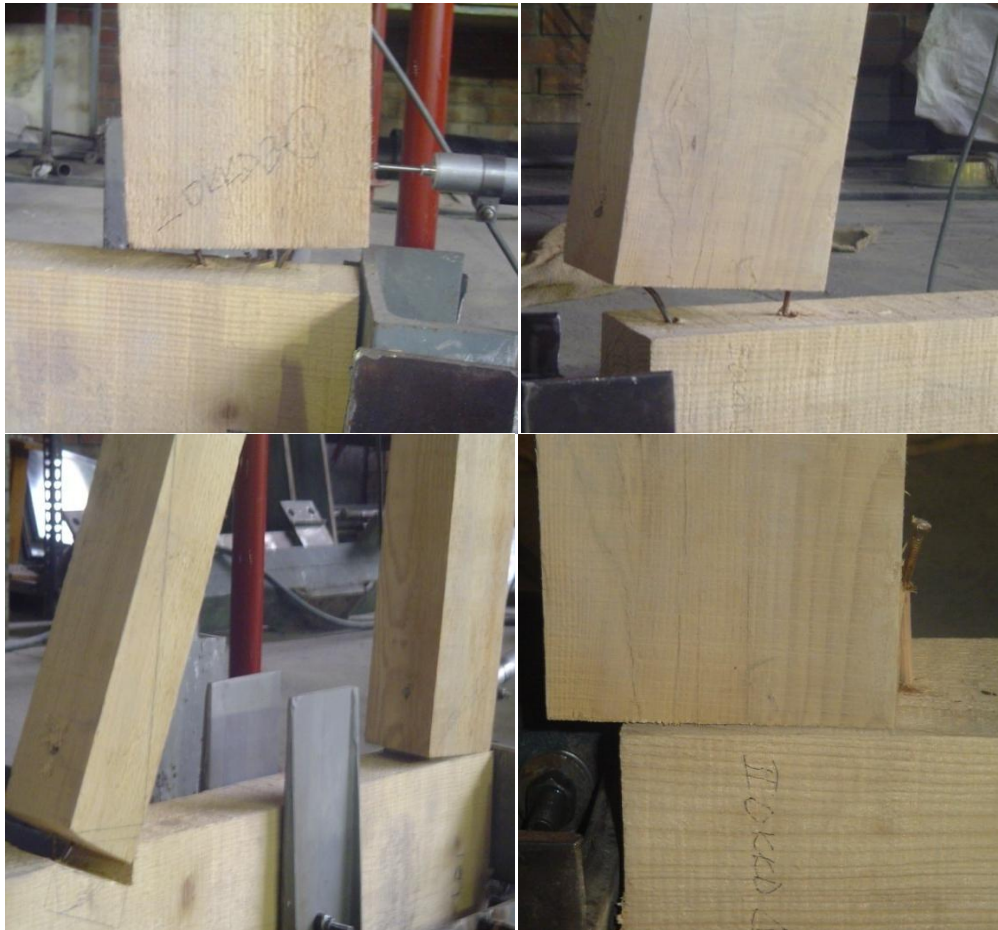
Figure 118: Examples to joint dilatation
