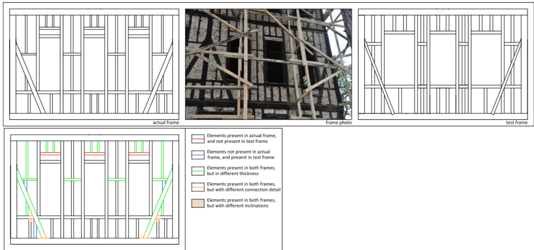
Figure 225: Drawings of actual frame and test Frame#6, showing the differences between them
