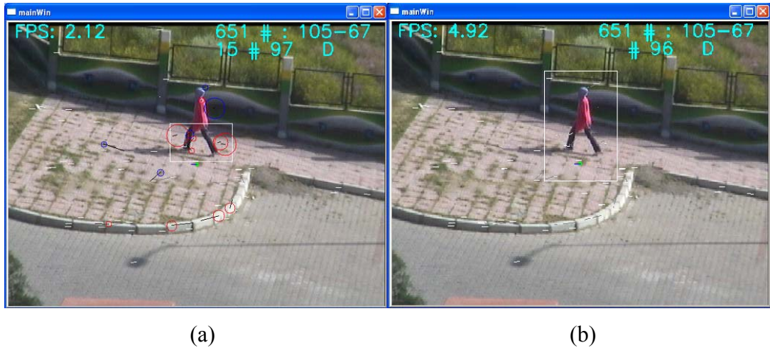
Figure 4-5 Outlier based detector, partially locates the object (a) while the object is located better with frame difference based detector (b)
