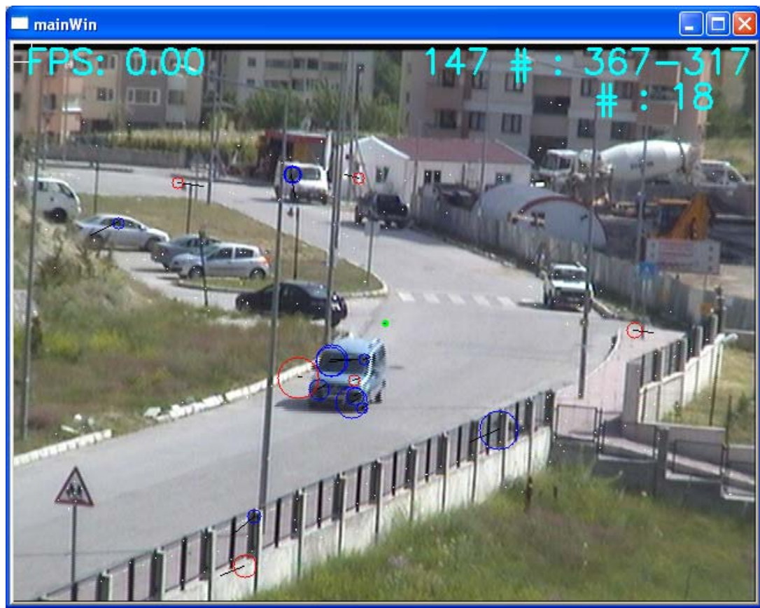
Figure 3-19 Inlier and outlier features on frame 147 of video1
