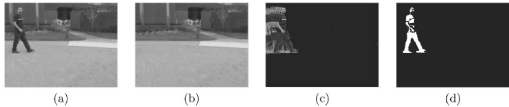
Figure 2-1 Background construction and foreground extraction example [4]
