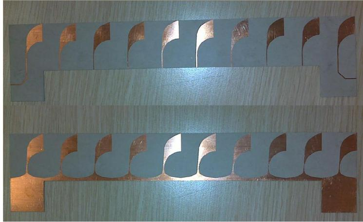
**Figure 6.9: Photograph of 10 element Antipodal Vivaldi Array**
