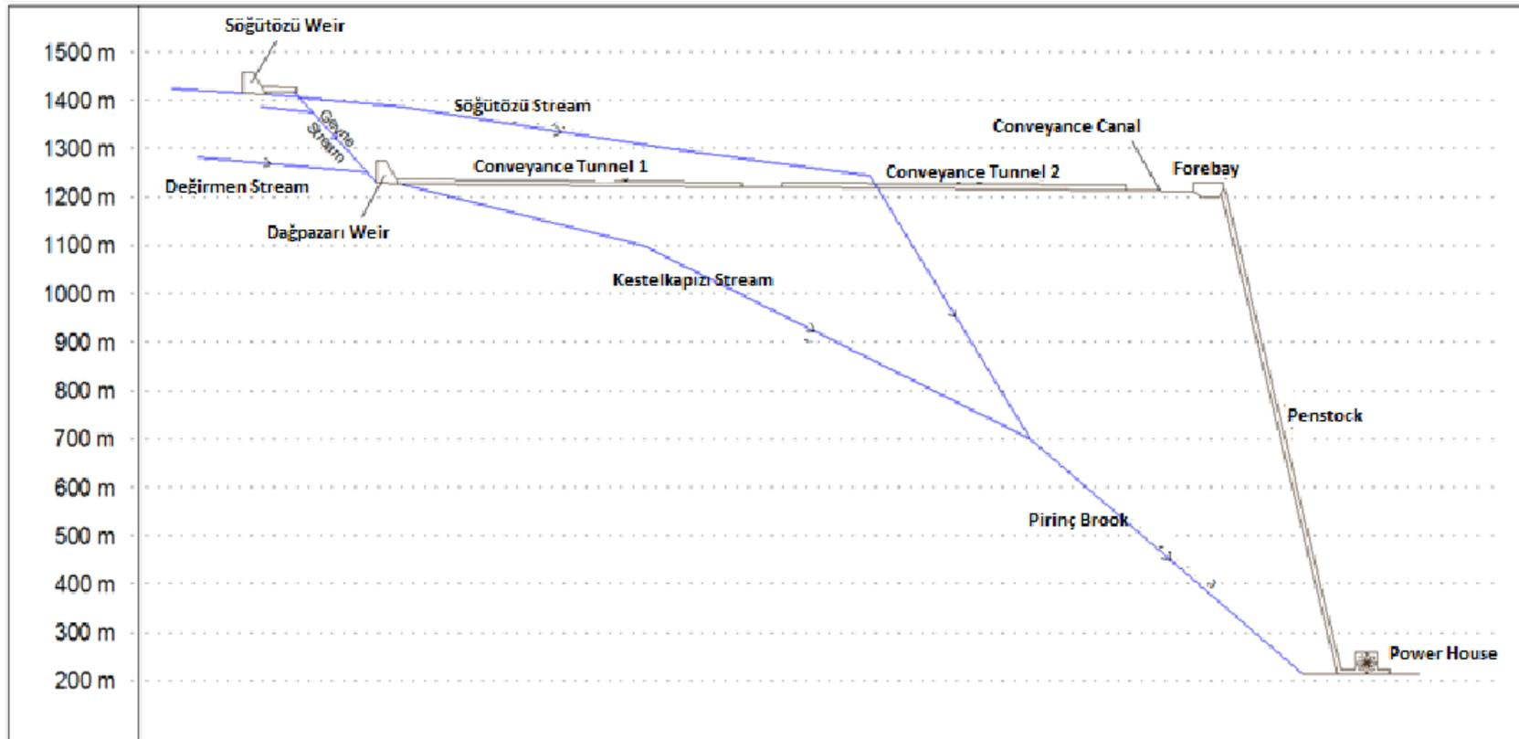
**Figure 3.5** Schematic description of Birkapılı HEPP facilities and creeks in the vicinity of the project site (profile)
