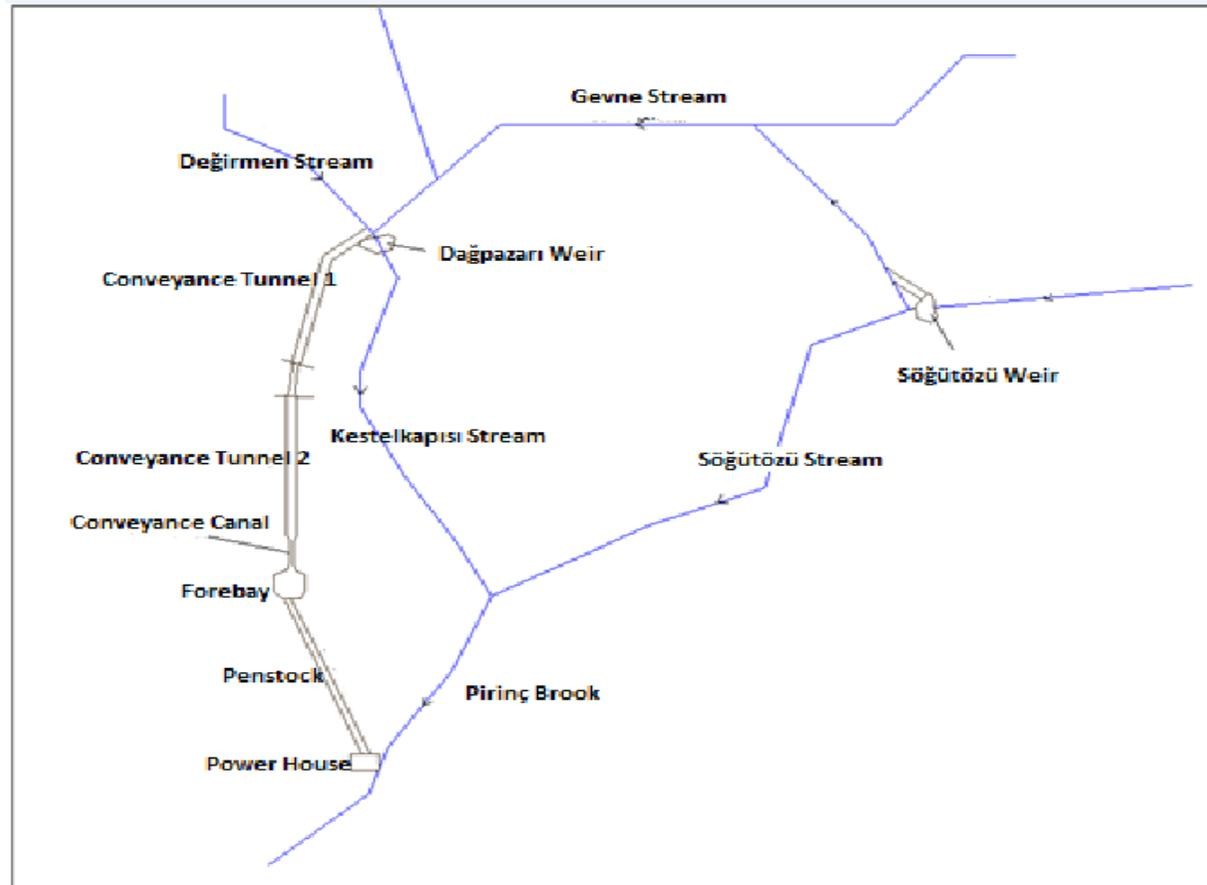
**Figure 3.4** Schematic description of Birkapılı HEPP facilities and creeks in the vicinity of the project site (plan)
