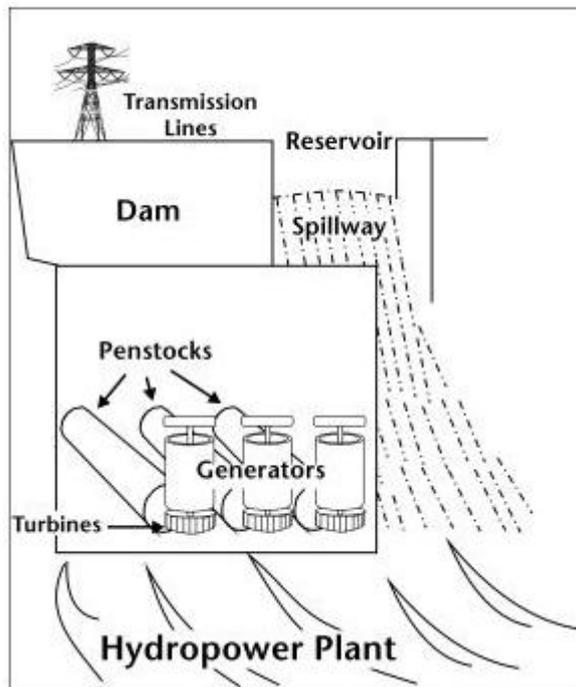
**Figure 2.1** Water cycle in a hydropower plant [25]
