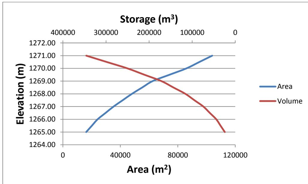
**Figure 4.1** Area-elevation-storage curves
