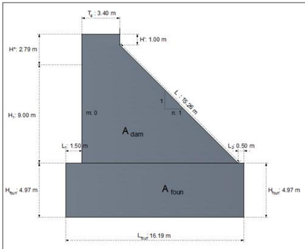
Figure A.1 Dam body cross-section
