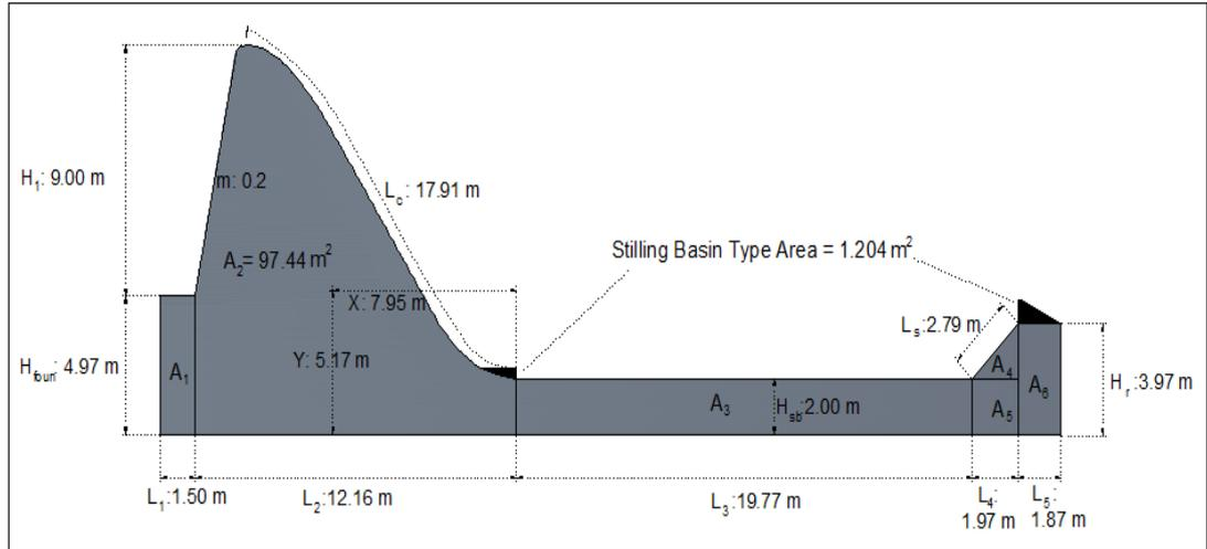
Figure A.2 Spillway cross-section
