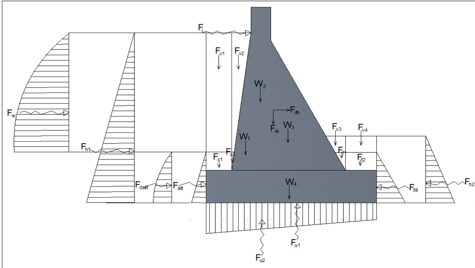
Figure 4.5 Forces developed on dam body
