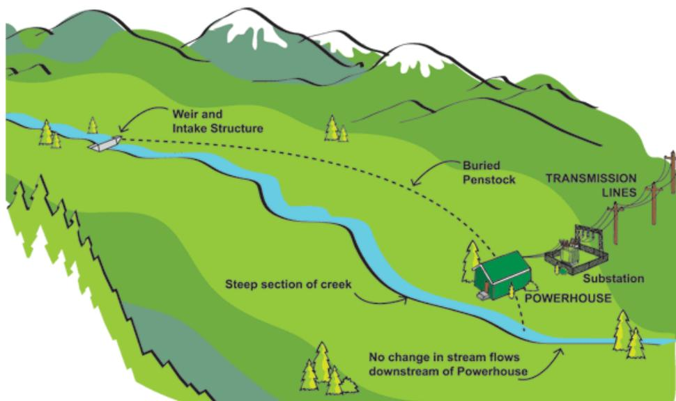
**Figure 2.2** Run-of-river hydroelectric power plants [27]
