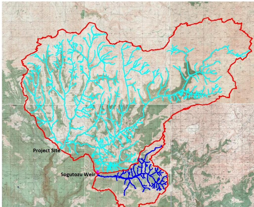
**Figure 4.4** Drainage area of the storage facility
