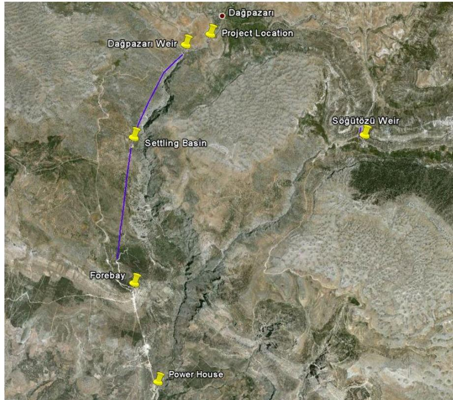
**Figure 3.3** The proposed location of the storage facility and existing facilities of Birkapılı HEPP
