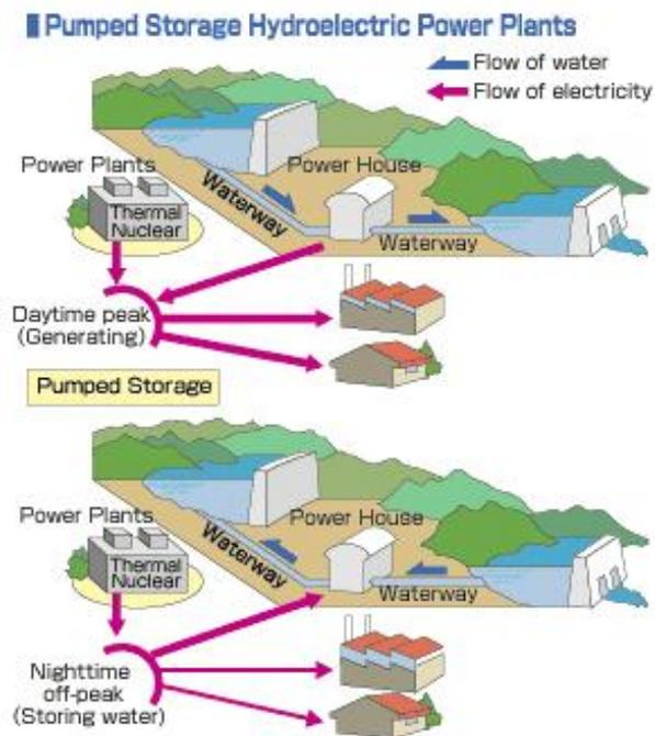
Figure 2.6 Working phases of a pumped-storage plant [33]
