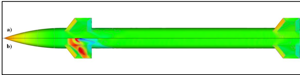
Figure 4-20: TCM-Surface Pressure Distribution, a) No jet, \alpha = 0^\circ b) C1, \alpha = 0^\circ , \dot{m} = 0.2 kg/s
