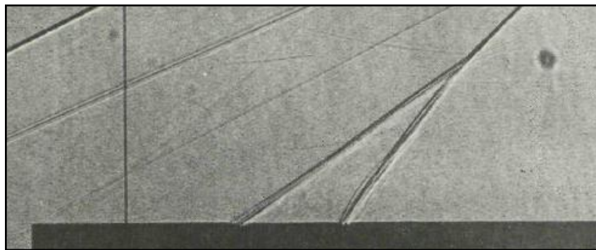
Figure 2-2: 2-D Flat Plate with Jet Injection Shadowgraph [26]
