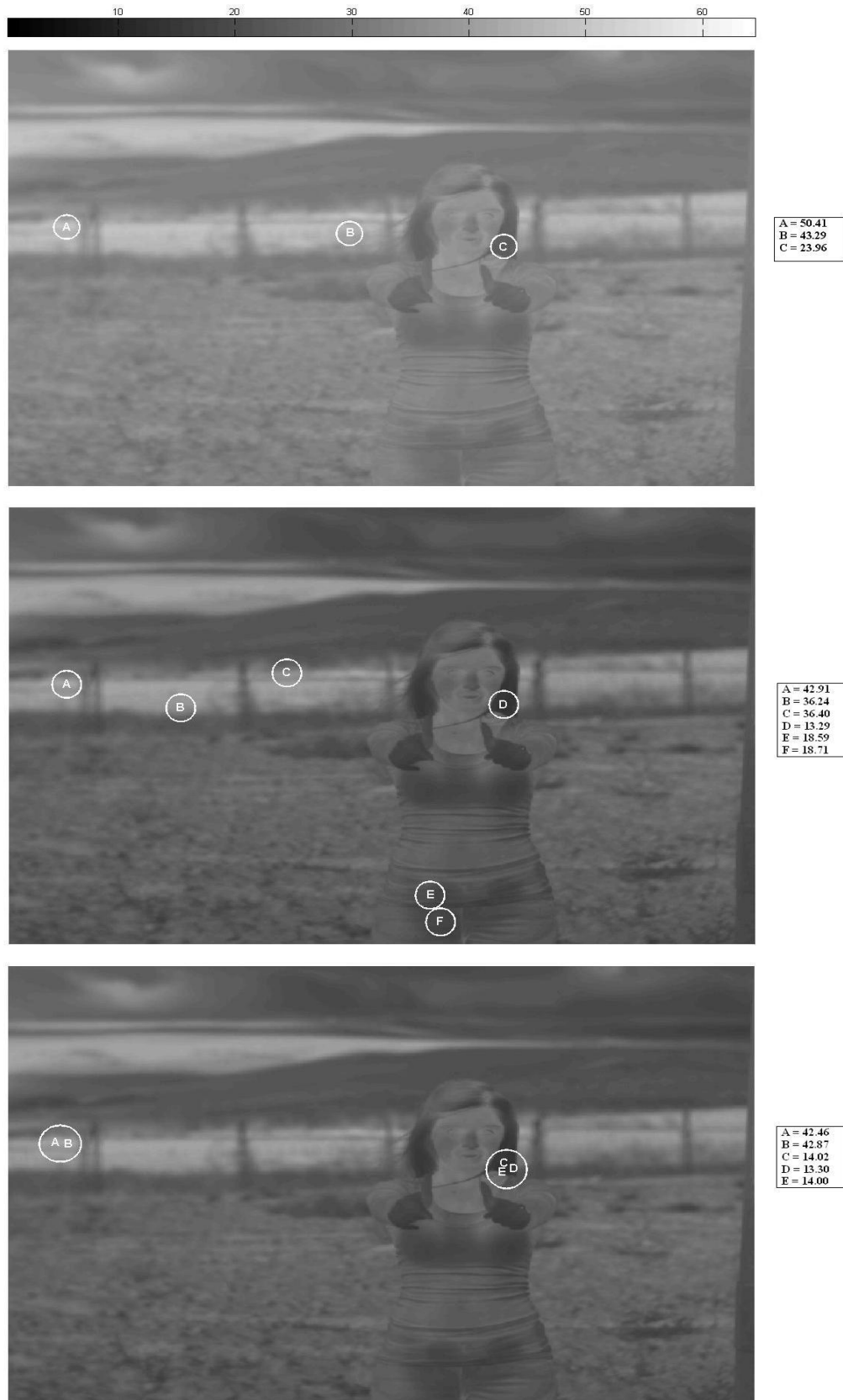
Figure 18 – Position of minimum and maximum errors in Frame 1 for Planck's Method (top panel), Curve Fit Method (middle panel), Lookup Table Method (bottom panel) All values are in °C.
