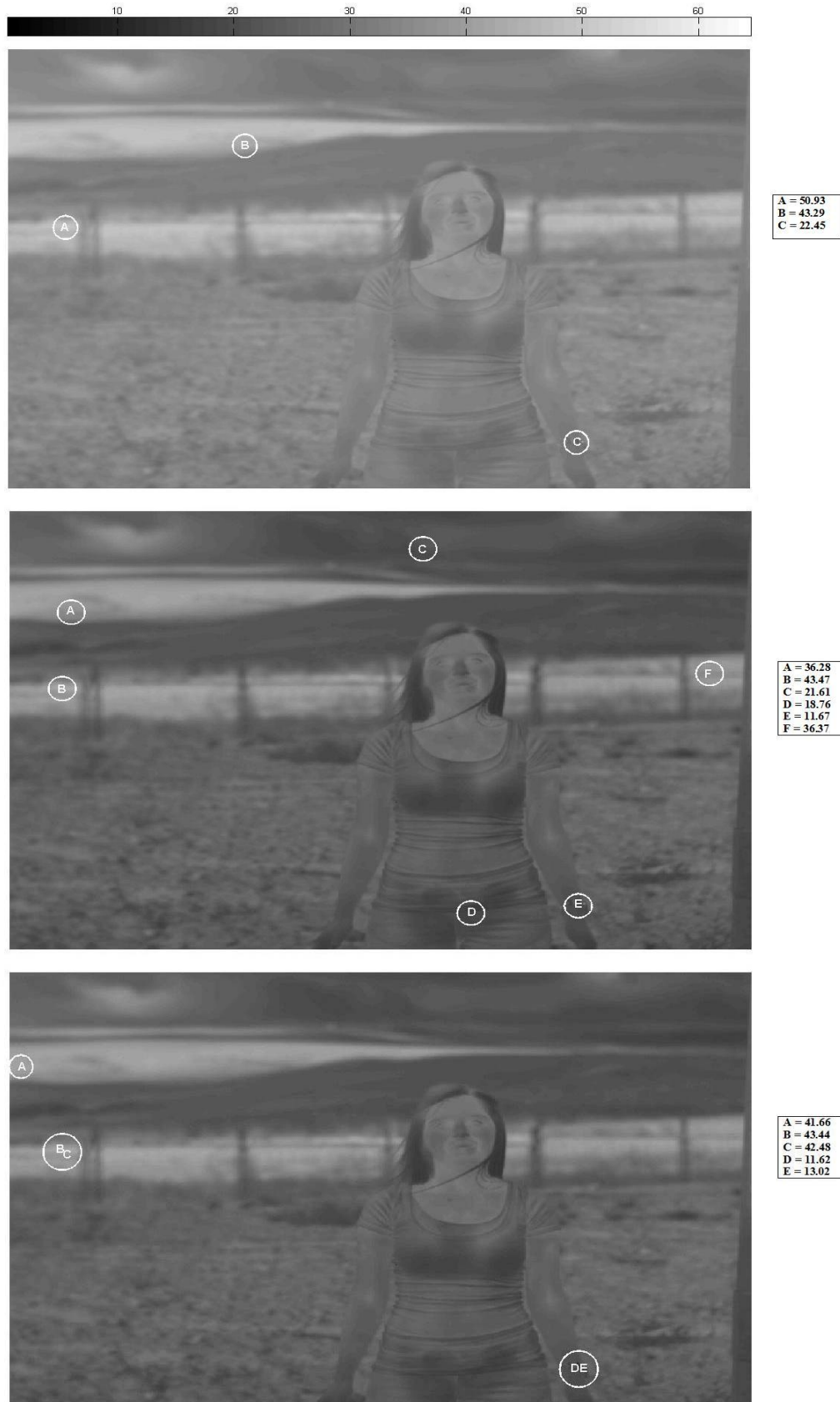
Figure 20 – Position of minimum and maximum errors in Frame 3 for Planck's Method (top panel), Curve Fit Method (middle panel), Lookup Table Method (bottom panel) All values are in °C.
