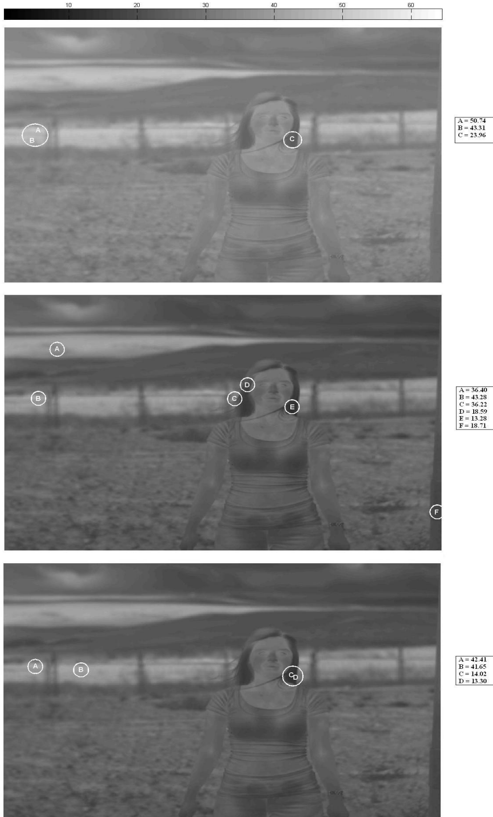
Figure 19 – Position of minimum and maximum errors in Frame 2 for Planck's Method (top panel), Curve Fit Method (middle panel), Lookup Table Method (bottom panel) All values are in °C.
