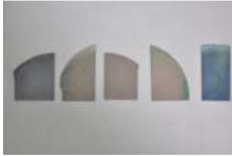
Figure 4.5.2 : The samples are lined up as 12 nm Ag film coated on surface textured Si, annealed at 200 °C, 300 °C, 400 °C and 500 °C, respectively.
