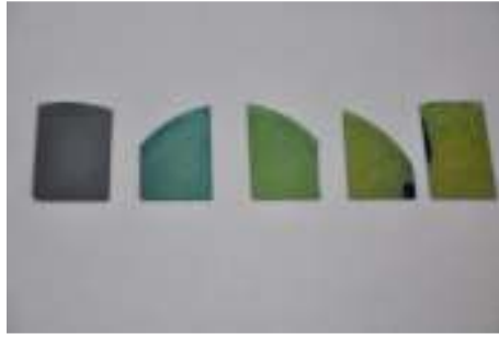
Figure 4.5.5 : The samples are lined up as 12 nm Ag film coated on surface textured Si with \text{Si}_3\text{N}_4 layer on it, annealed at 200 °C, 300 °C, 400 °C and 500 °C, respectively.
