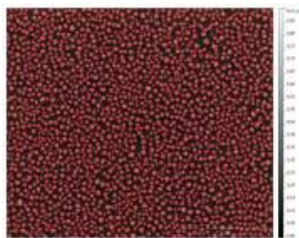
Figure 3.1.5 : A representative SEM image after masking the nanoparticles
