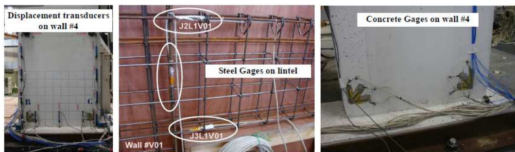
Figure 2-10 Examples of local instrumentation of SMART specimen
