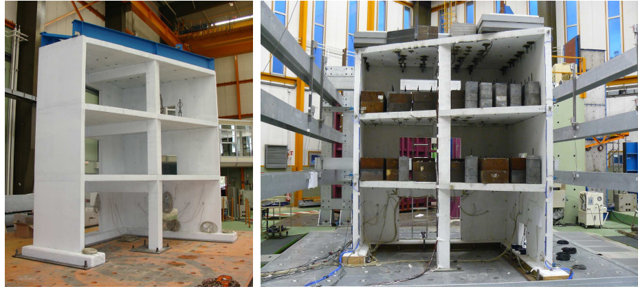
Figure 2-9 SMART Specimen, unloaded and fully loaded (Lermitte et al., 2008)
