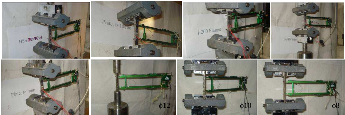
Figure A2.10 Pictures of the coupon specimens
