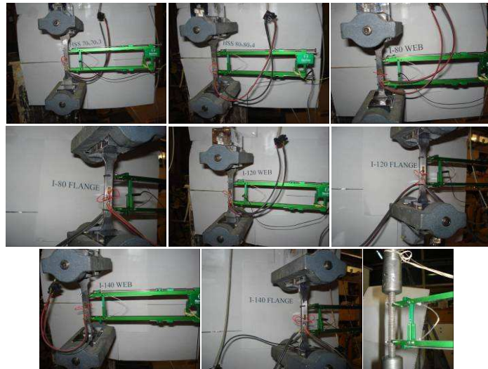
Figure A1.16 Pictures of the coupon tests (from left to right HSS70x70x3, HSS 80x80x4, I-80 web, I-80 flange, I-120 web, I-120 flange, I-140 web, I-140 flange, \phi 12 )
