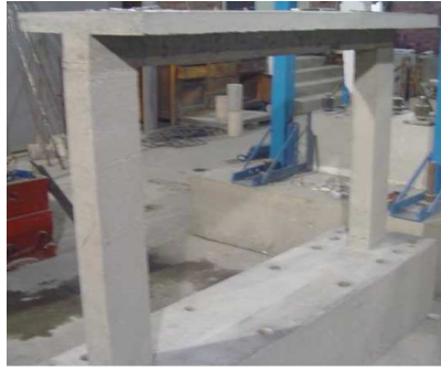
Figure A1.5 RC frame after removing the molds
