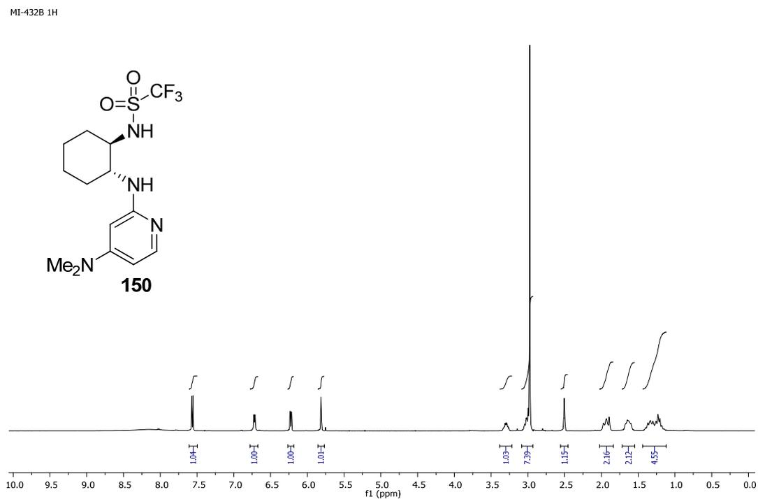
**Figure A13.**  $^1\text{H}$  NMR spectrum of **150**
