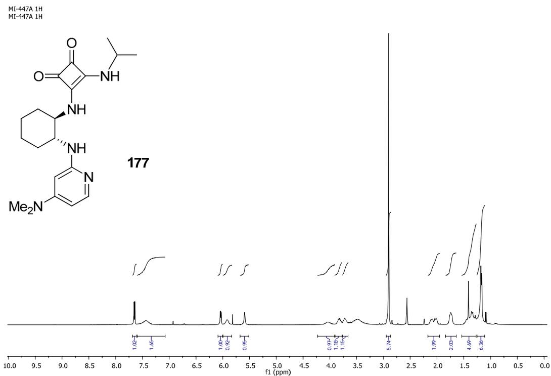
Figure A 41.  $^1\text{H}$  NMR spectrum of **177**
