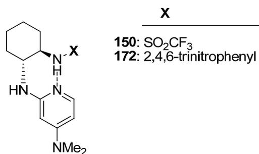
**Figure 11.** Intramolecular H-bond lowering activity of catalysts **150** and **172**
