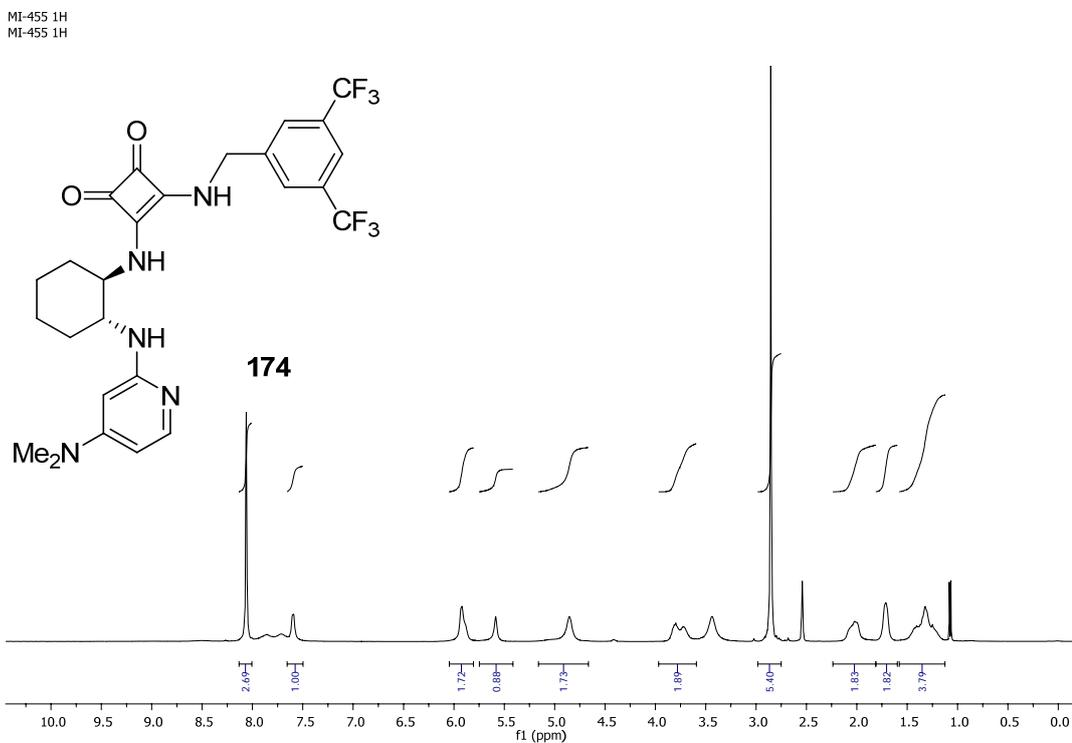
Figure A35.  $^1\text{H}$  NMR spectrum of **174**
