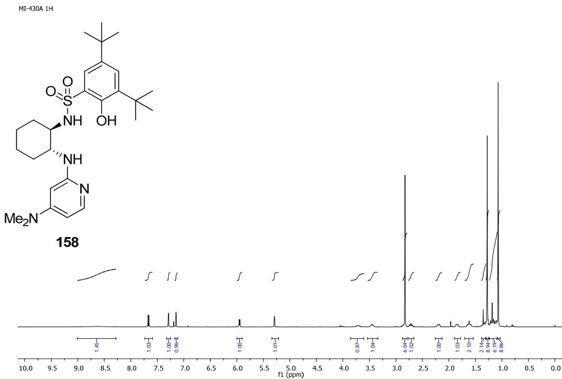
Figure A27. <sup>1</sup>H NMR spectrum of **158**
