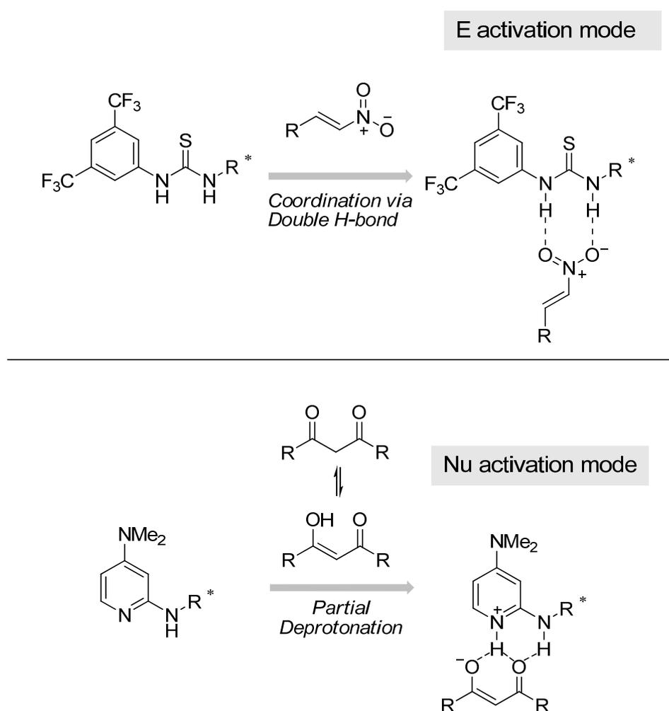
**Figure 9.** Proposed nucleophile and electrophile activation modes by active catalytic units of **130**
