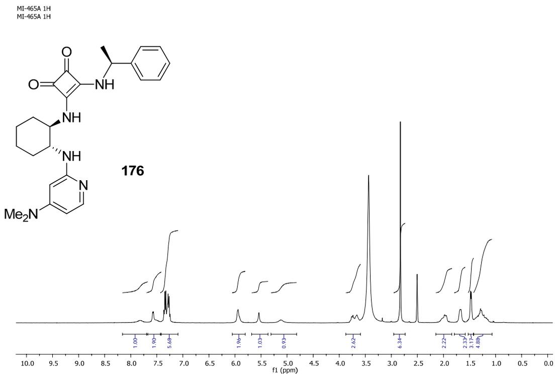
Figure A39.  $^1\text{H}$  NMR spectrum of **176**
