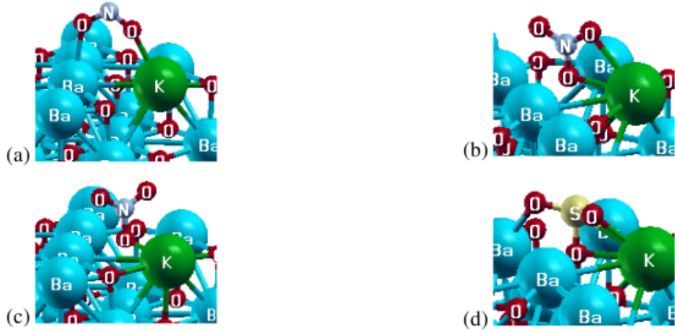
Figure 3.6: Optimized adsorption geometries of \text{NO}_2 on K-doped BaO (100) surface: (a) Bridge, (b) Tilted, (c) N-down II. Optimized adsorption geometry of \text{SO}_2 on K-doped BaO (100) surface: (d) S-down.
