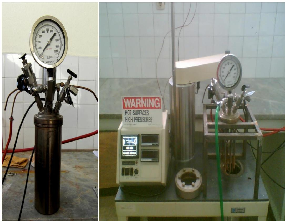
Figure 12. The autoclave used in HPAL experiments (Titanium-grade 4).
