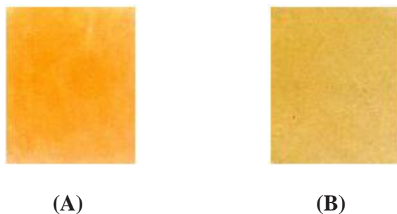
Figure 3.18 ERL4221E/ \text{Ph}_2\text{I}^+\text{PF}_6^- /PHEHT mixture (A) before exposure to solar irradiation, (B) after 5 minutes of irradiation.
