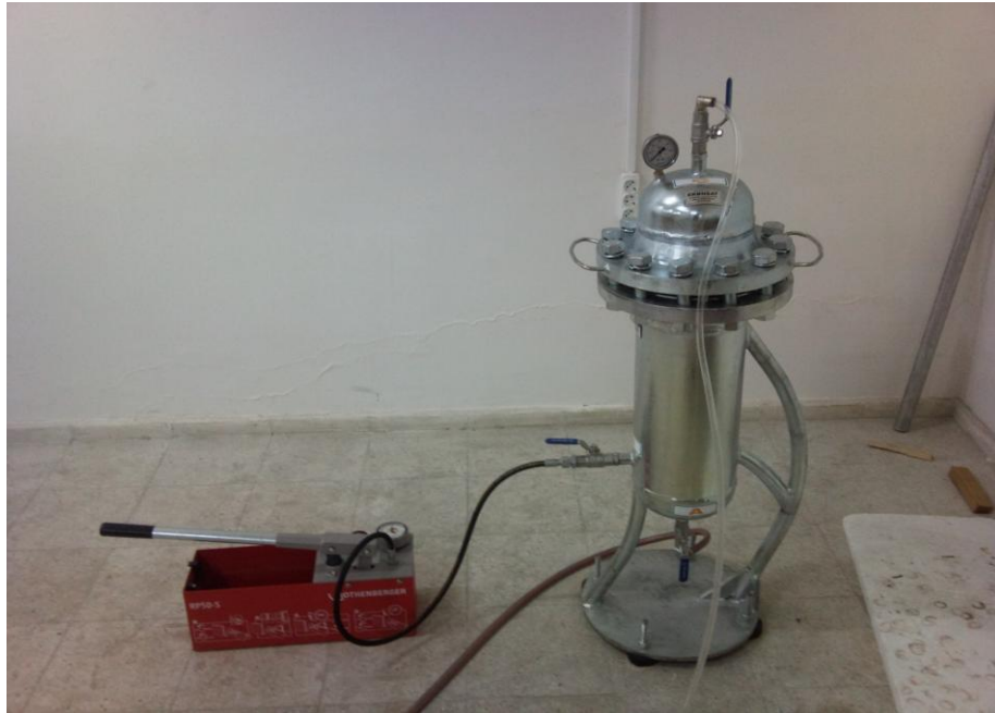
Figure 3.64: Photograph of the pressure tank used in the mechanical test
