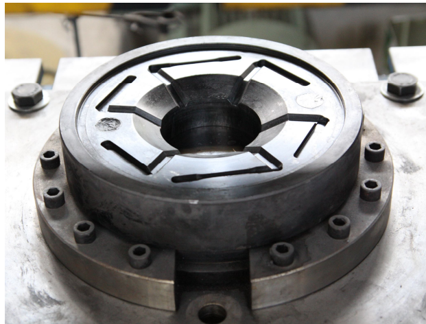
Figure 3. 2 The hot worked tool steel die is designed for two tensile specimens and four bending specimens
