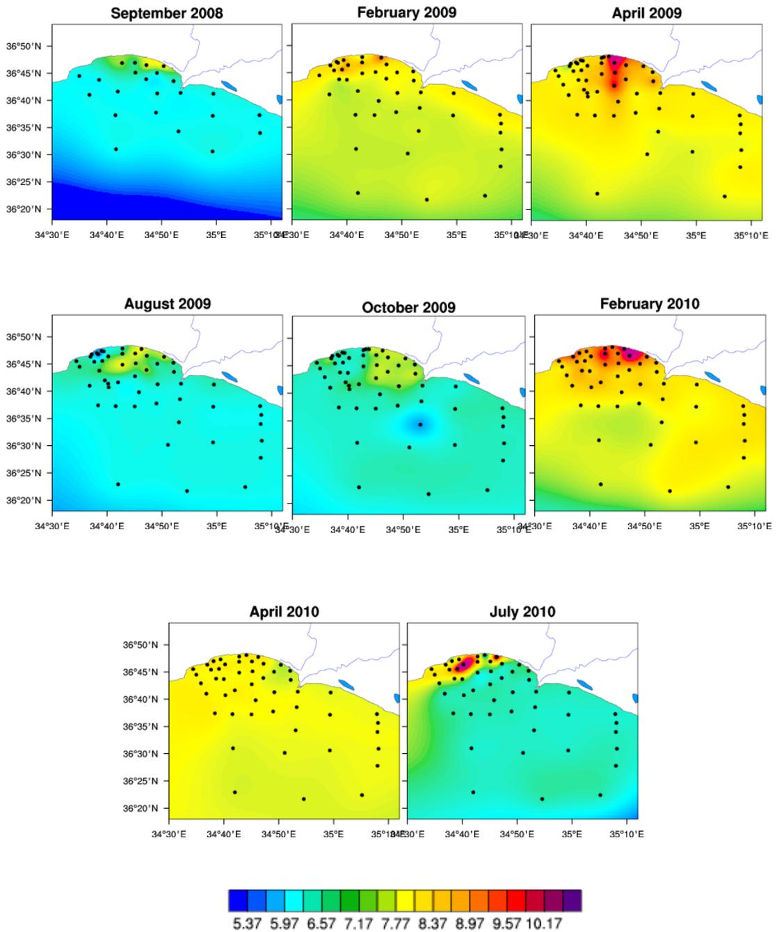
Figure 3.46. Changes in surface dissolved oxygen concentrations (all drawn at a constant scale; 5.37 – 10.27 mg/l) in Mersin Bay.
