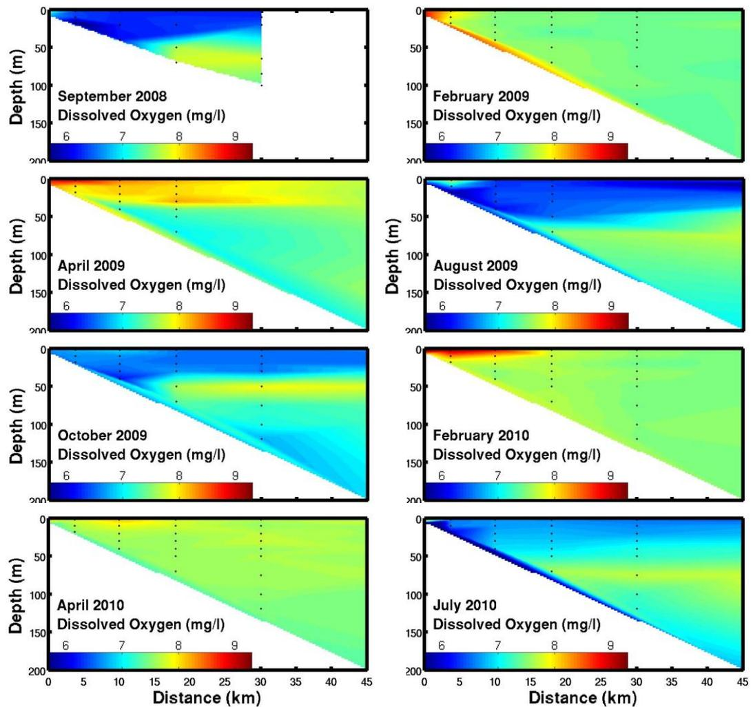
Figure 3.47. Observed dissolved oxygen profiles (all drawn at a constant scale; 5.7 – 9.3  $\mu\text{M}$ ) in Mersin Bay.
