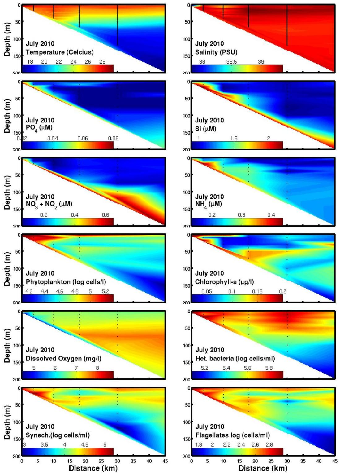
Figure 3.23. Vertical distributions of physical, biological and chemical parameters in July 2010.
