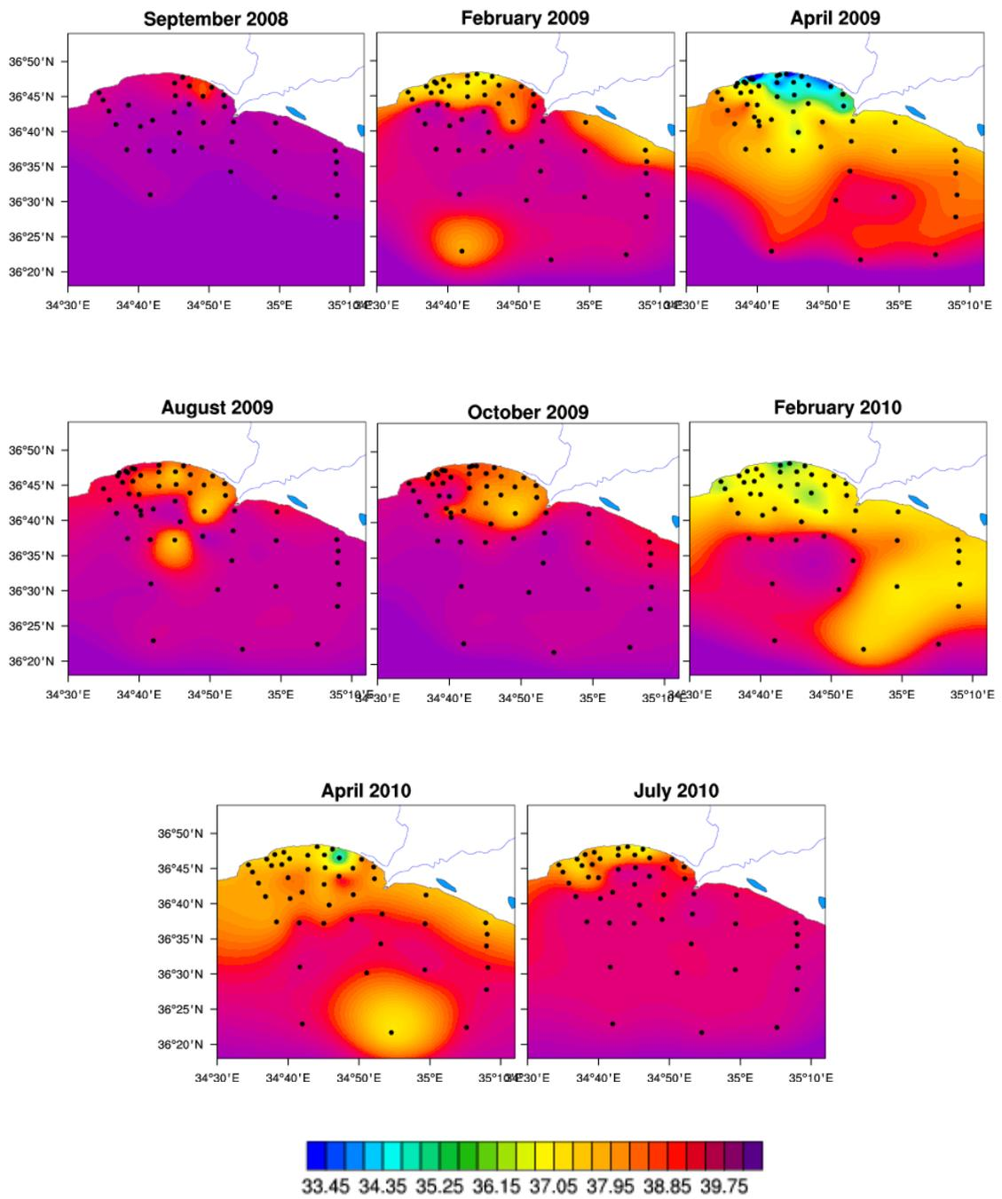
Figure 3.28. Changes in surface salinity (all drawn at a constant scale; 33.45 - 39.84 PSU) in Mersin Bay.
