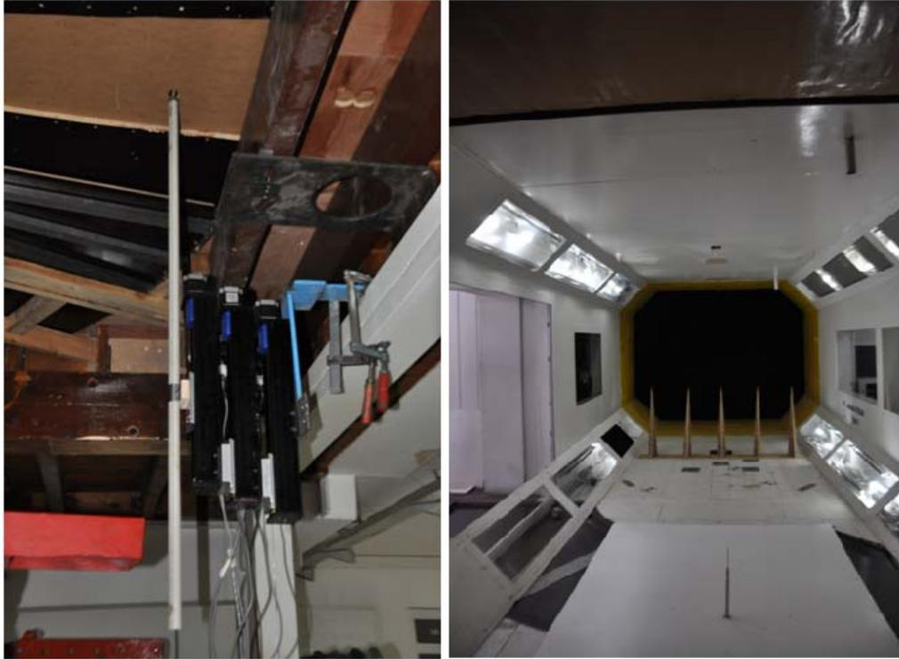
**Figure 3.8 Photographs of the traverse system and hot wire anemometer system taken during the test**
