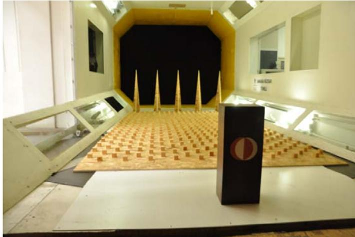
**Figure 4.2 Alignment of the model in test section**
