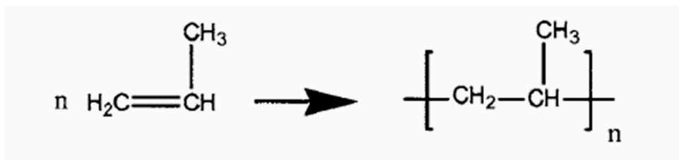
Figure 2.1 Synthesis of Polypropylene [15]
