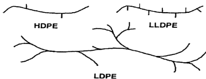
Figure 2.4 Structures of HDPE, LLDPE and LDPE [15]
