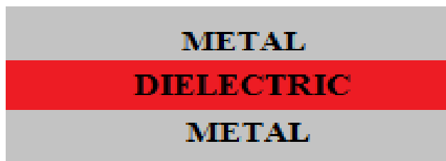
Figure 3.18 MIM structure for dielectric measurements
