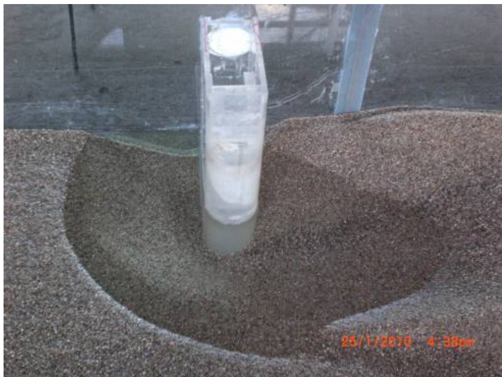
Figure 2.2 General view of the scour hole around a semi-circular end abutment tested in this study
