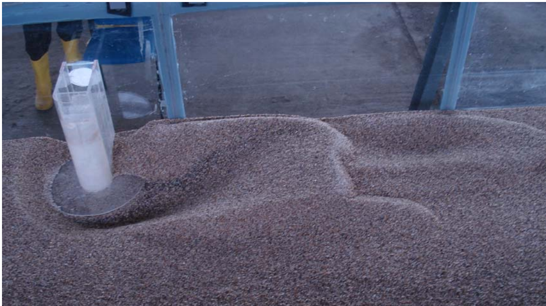
Figure 4.2 Abutment L_a=20 cm with collar B_c=10 cm at Z_c/y=-0.25
