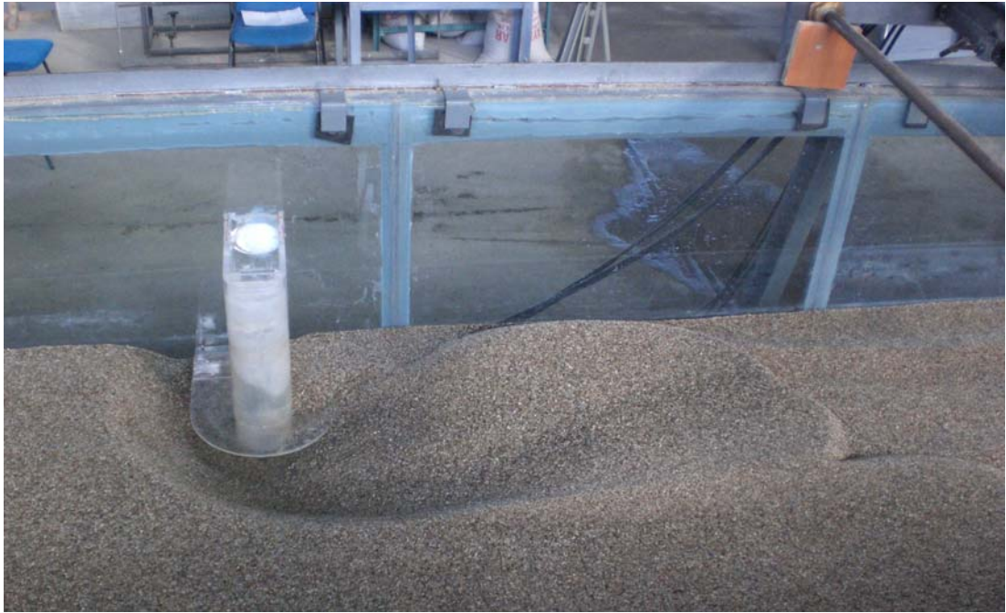
Figure 4.5 Abutment L_a=25 cm with collar B_c=7.5 cm at Z_c/y=-0.25
