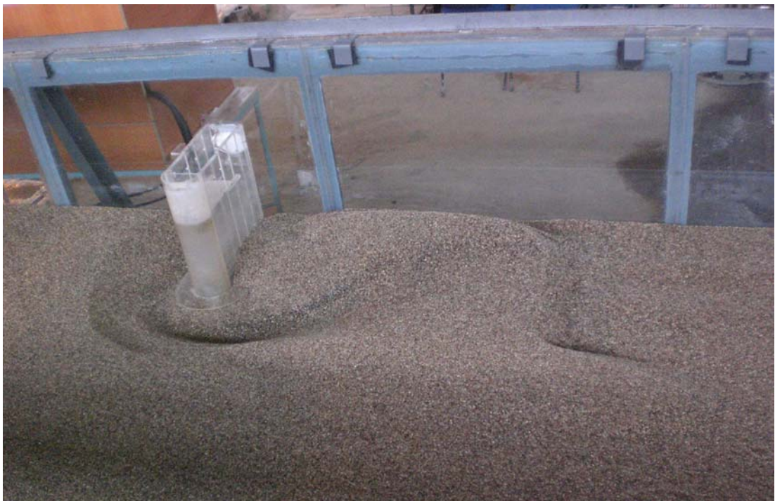
Figure 4.6 Abutment L_a=30 cm with collar B_c=5.0 cm at Z_c/y=-0.50
