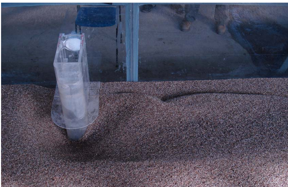
Figure 4.4 Abutment L_a=25 cm with collar B_c=5 cm at Z_c/y=0
