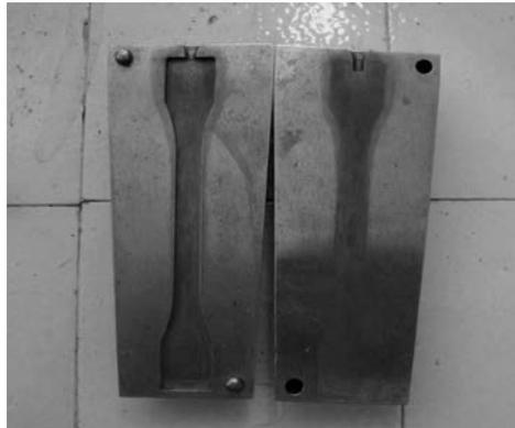
Figure 3-24 The mold in Daga micro injection machine
