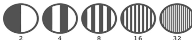
Figure 2-32 Static mixers with different number of flow divisions (striations)
