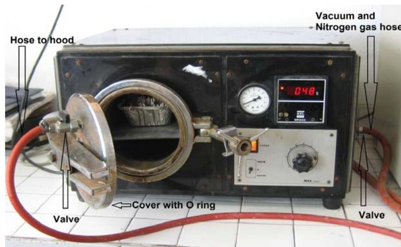
Figure 3-18 Vacuum oven for sample drying
