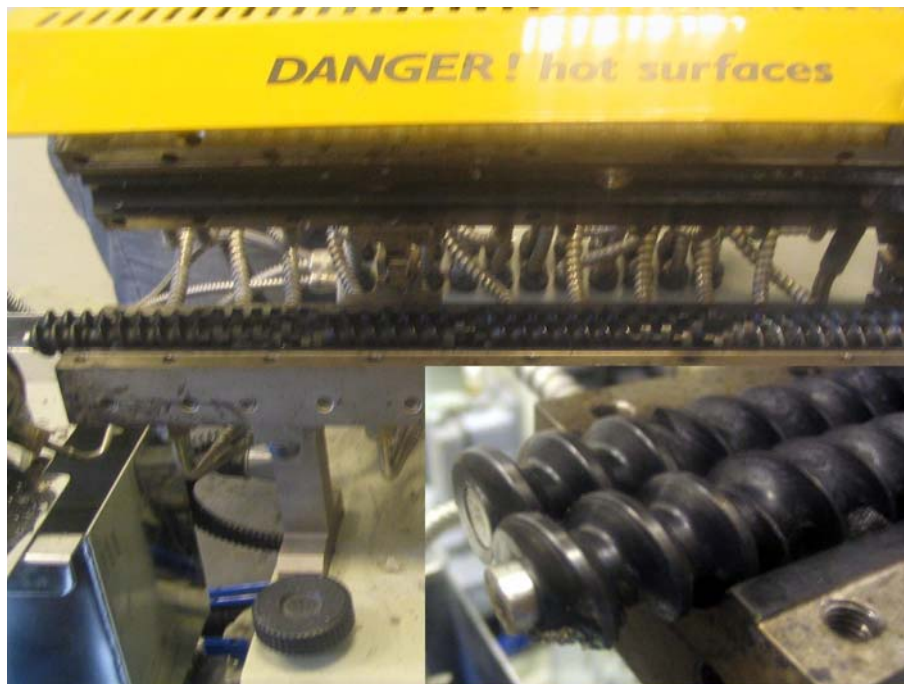
Figure 3.9 Screw Configuration of Thermo Prism TSE 16 TC twin screw extruder
