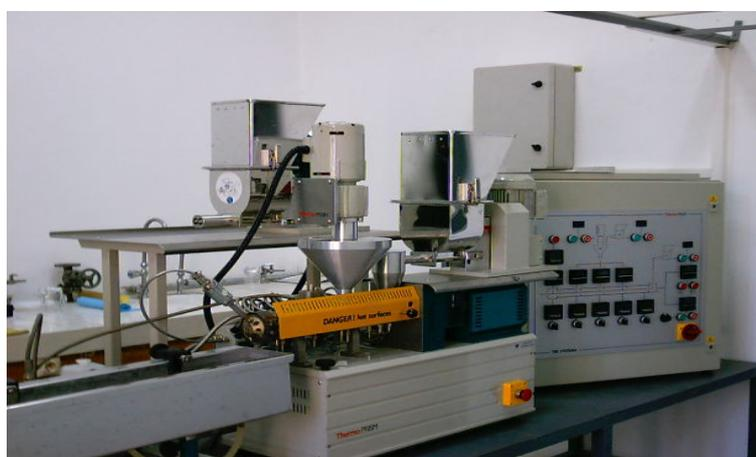
**Figure 3.6** Thermo Prism TSE 16 TC twin screw extruder
