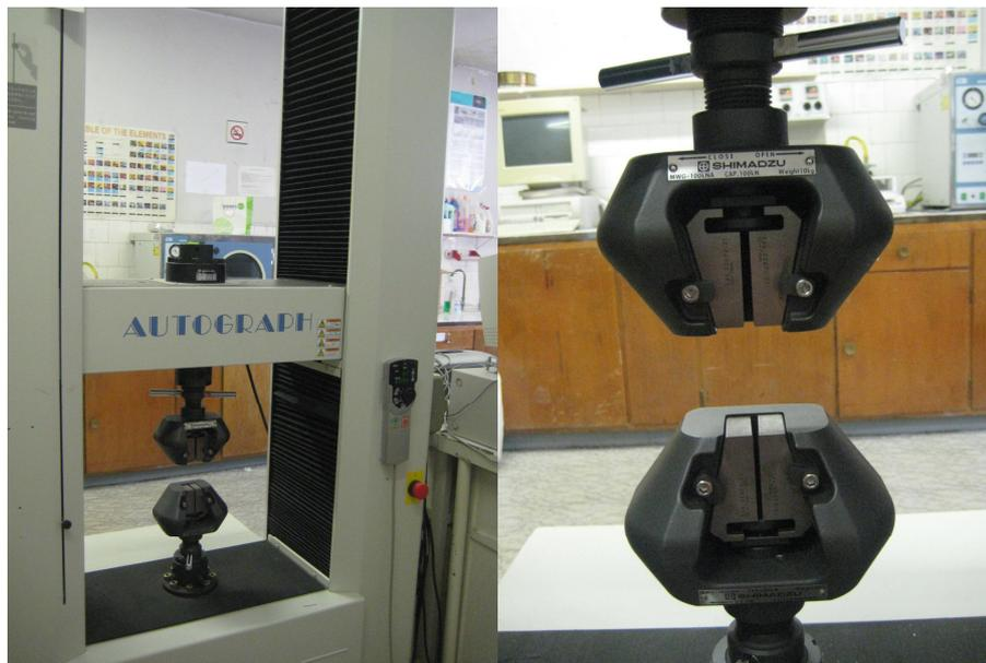
**Figure 3.12** Shimadzu AG-IS 100 kN test machine
