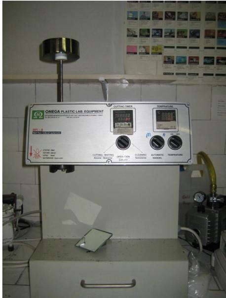
**Figure 3.11** Omega Melt Flow Indexer
