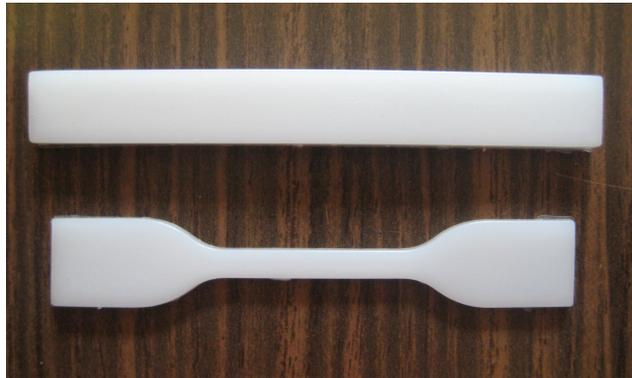
**Figure 3.9** A photograph of injected molded HDPE
