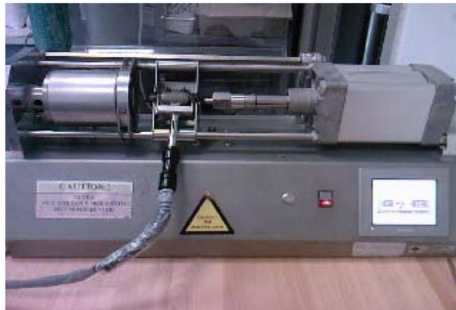
**Figure 3.7** Injection molding equipment.
