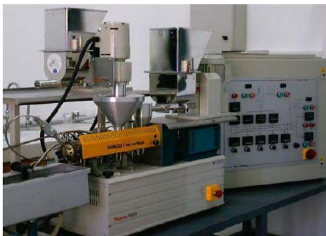
**Figure 3.4** Thermoprism TSE 16 TC twin-screw extruder.
