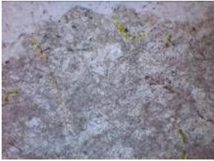
**Figure 3.23** View of a karstic vein and green biological activity on the exterior surface of a deteriorated sample from the West Terrace. (20X cross nicols)
