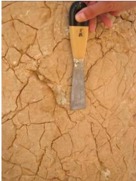
**Figure 3.6** Material losses by dissolution of limestone through karstic veins on the head of Kommagene at the west terrace of Nemrut Dağ Monument
