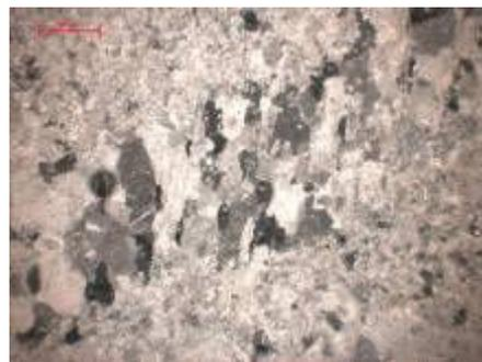
**Figure 3.16** View of a Karstic vein in Nemrut quarry limestone, scale bar: 100  $\mu$
