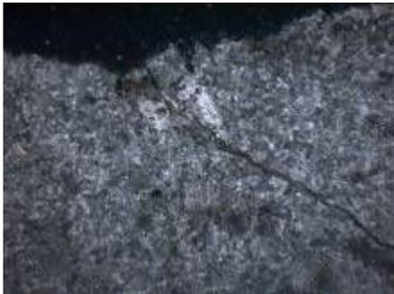
**Figure 3.25** View of a crack and biological activity on the exterior surface of a deteriorated sample from the West Terrace. (20X cross nicols)
