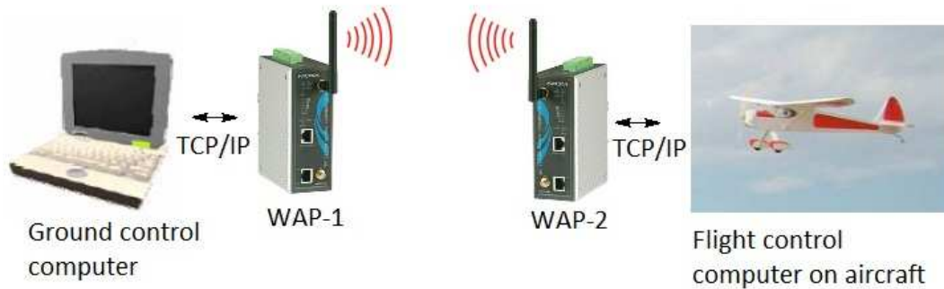
Figure 2.21: Air-ground Communication Using Wireless Access Points
