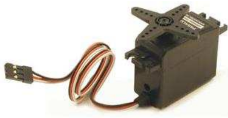
Figure 2.14: Standard Analog RC Servo
