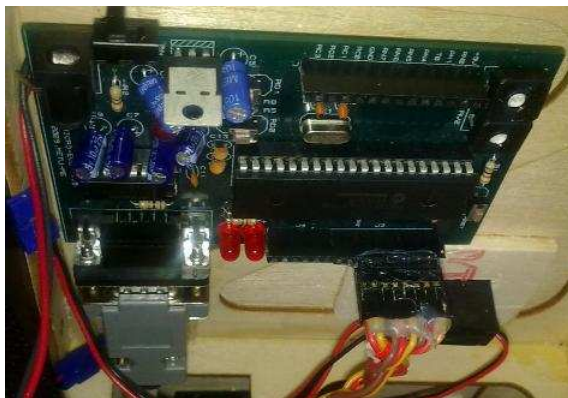
Figure 2.18: Servo Driver Board Mounted Inside the Airplane
