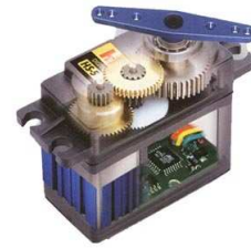
Figure 2.15: RC Servo (inside)
