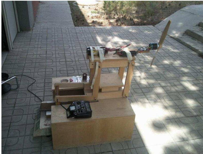
Figure 2.29: Motor Test Setup
