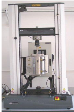
Figure 3.2 Instron 3367 Creep Tester with split furnace and chamber facilities.
