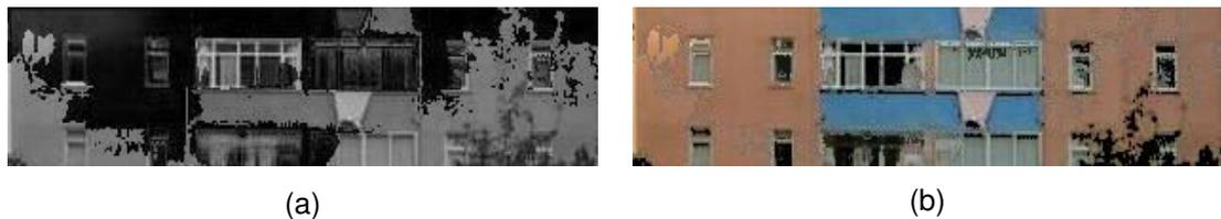
Figure 5.39. (a) The grayscale difference image, in which dark areas refer to minor or no change and (b) the updated candidate image.
