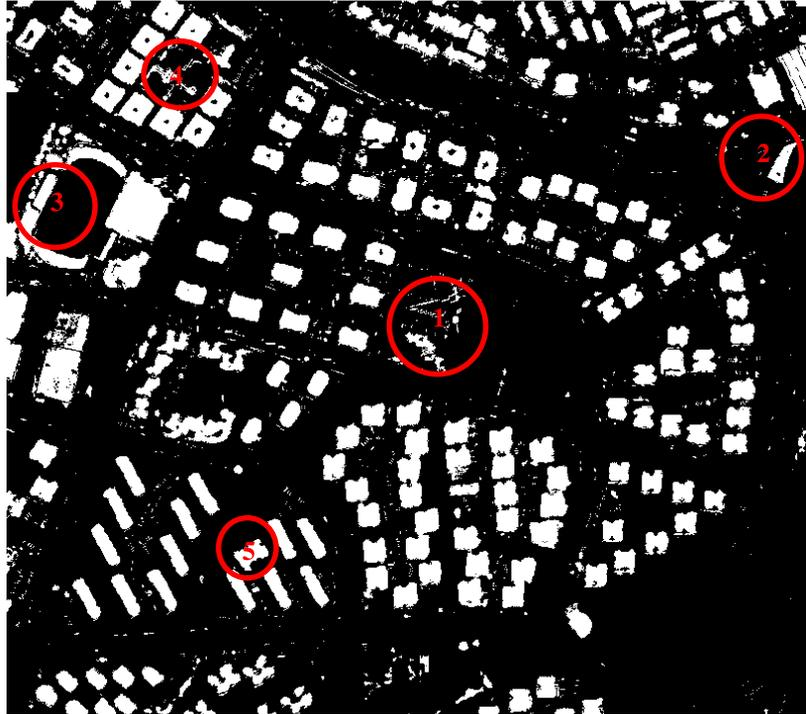
Figure 7.3. The building regions extracted using the proposed adaptive fuzzy-genetic classification approach with the approximate fitness value of **83**.
