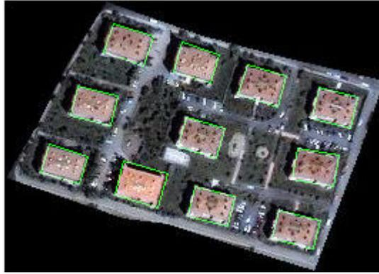
Figure 4.23. The extracted building footprints overlaid with the image.
