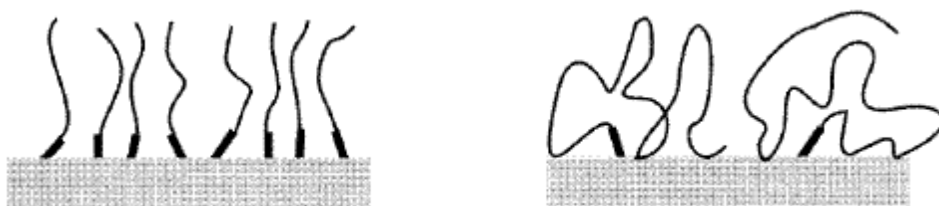
Figure 64 Schematic representation of thiol modified short and long oligonucleotides behavior onto the gold surface (Steel, Levicky, Herne, & Tarlov, 2000).
