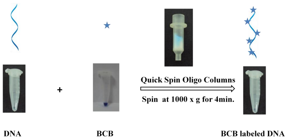
Figure 20 Schematic representation of noncovalent labeling of DNA with BCB.
