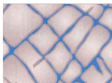
b) In hard rock, groundwater can be transmitted through fissures or fractures. If the primary porosity is small groundwater flow is virtually restricted to fissures.
