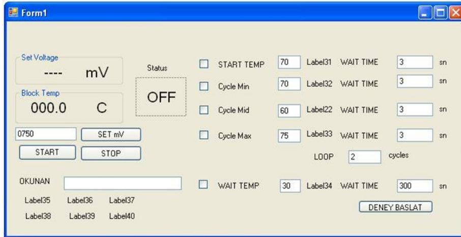
**Figure 3.27** The software of thermal cycler for computer
