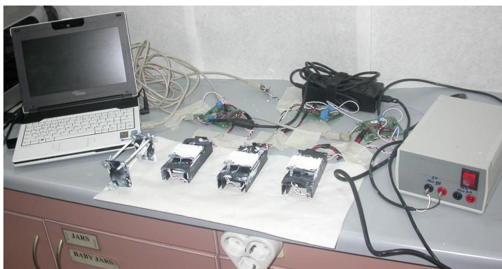
**Figure 3.35** The prototype of capillary thermal cycler
