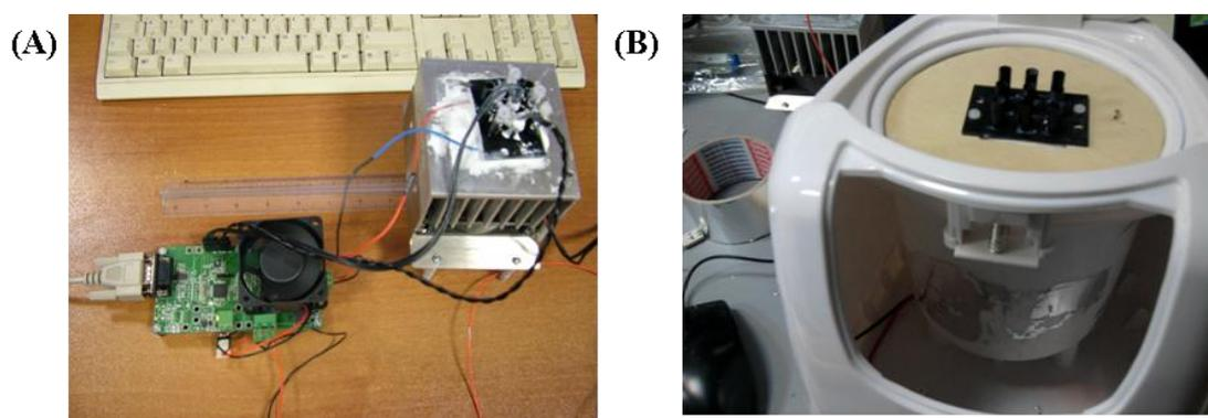
**Figure 3.26** The second prototype of newly developed conventional thermal cycler
