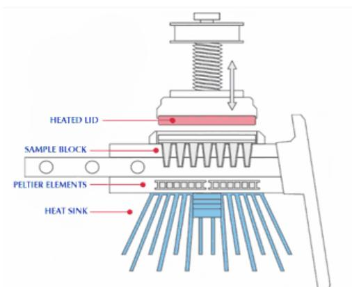
**Figure 1.8** Schematic representation of thermal cycler that is cooled by Peltier system ([http://www.dharmacon.com/uploadedImages/Home/Products/PCR\\_Research\\_Products/PCR\\_Instruments/Piko\\_Thermal\\_Cycler/HEATPUMP.gif](http://www.dharmacon.com/uploadedImages/Home/Products/PCR_Research_Products/PCR_Instruments/Piko_Thermal_Cycler/HEATPUMP.gif))
