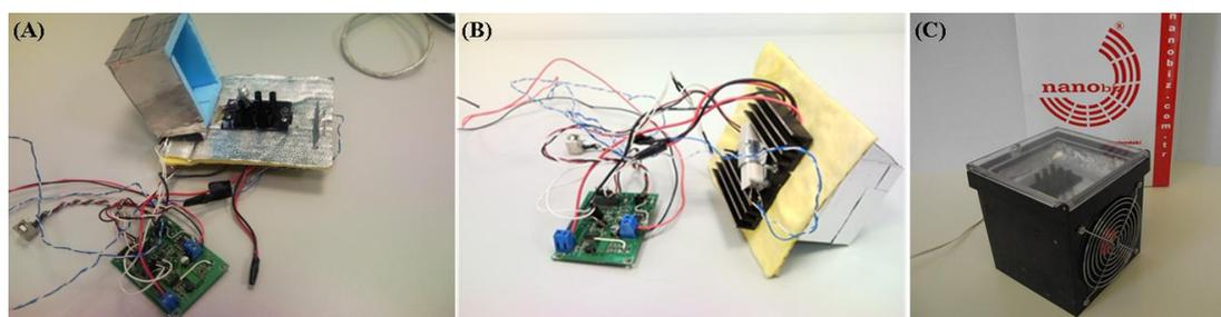
**Figure 3.24** The first prototype of newly developed conventional thermal cycler
