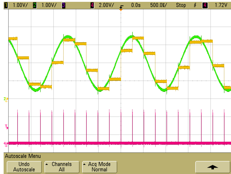
Figure 3.17: Test results of the sample-and-hold block. The block can successfully store signals between 0.5-3.5V.
