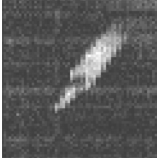
Figure 1.4: An image of hot soldering iron taken with the 64x64 SOI-CMOS microbolometer implemented with XFAB SOI-CMOS technology in METU.
