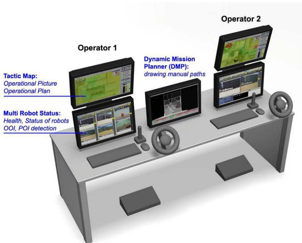
Figure 18 Representative Drawing of the Ground Control Station (GCS) Monitors with their Corresponding Functions
