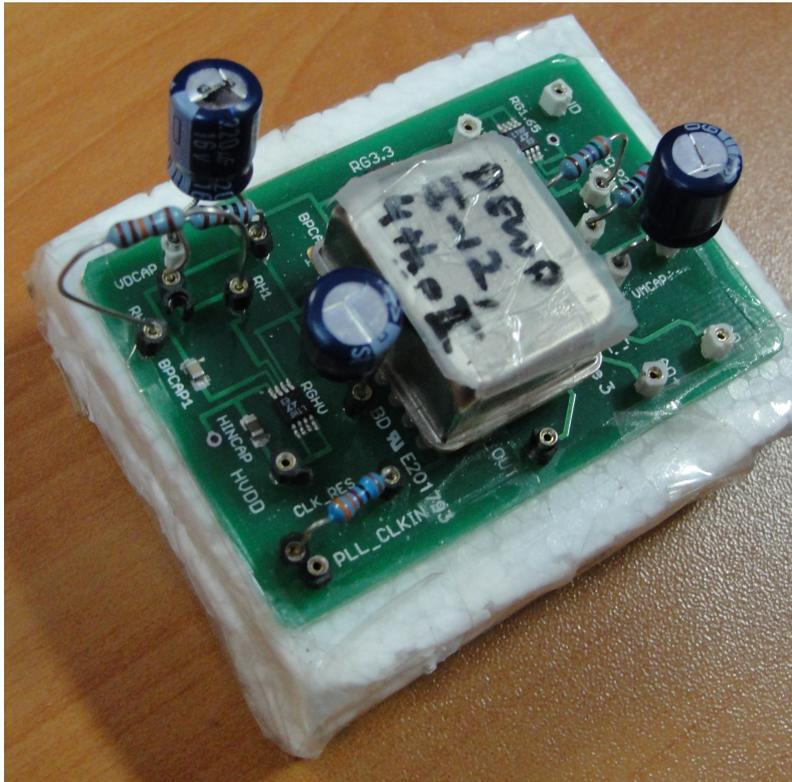
Figure 5.5: Photo of the test system with interface PCB and hybrid accelerometer package.
