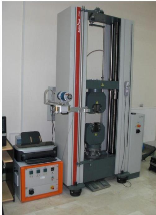
**Figure 4.2:** Zwick/ Roell Z300E All-round Universal Testing Machine
