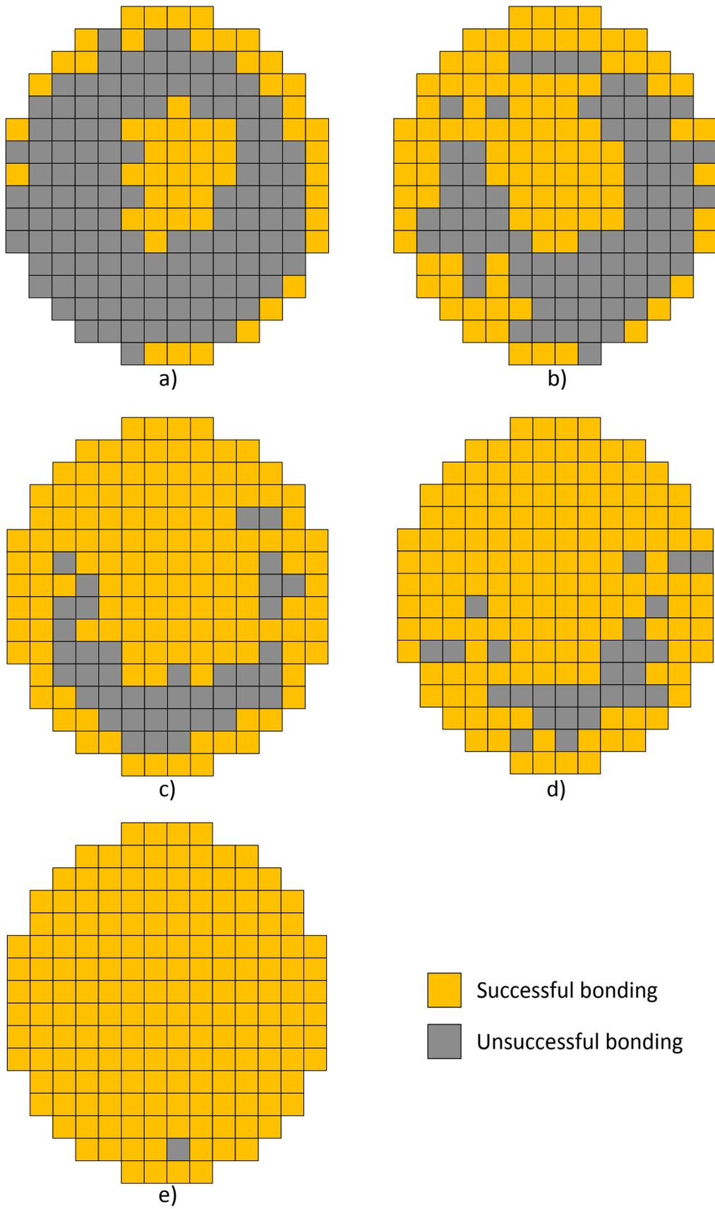
Figure 3.12: The uniformity results of glass frit bonds on glass wafer with lateral feedthroughs: (a) bond#1, (b) bond#2, (c) bond#3, (d) bond#4, and (e) bond#5.
