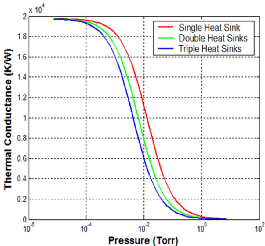
Figure 2.14: The effect of heat sinks on the pirani gauge performance.
