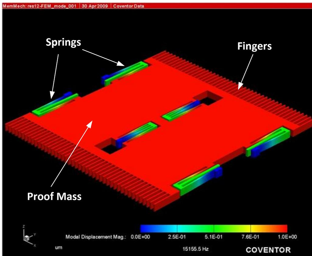
Figure 2.6: First mode of Design-2 at 15.1 kHz. The estimated frequency is 15 kHz, which is close to the simulation result.
