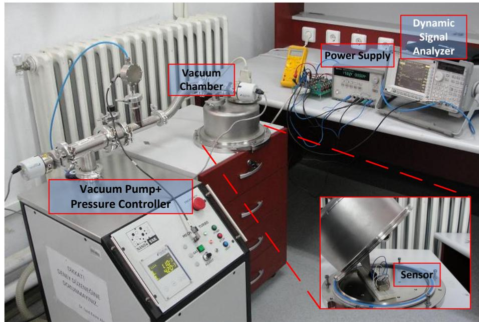
Figure 4.3: The vacuum test setup for gyroscopes and resonators.
