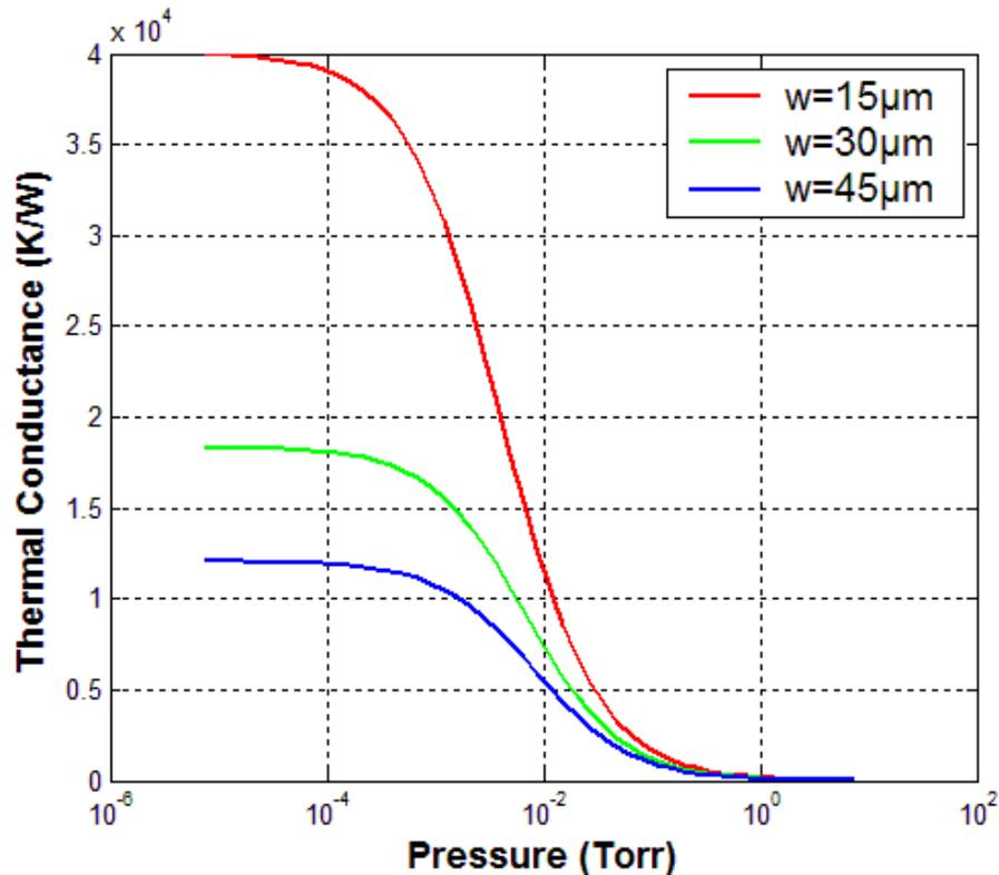
Figure 2.11: The effect of resistor width on the performance of a pirani gauge.
