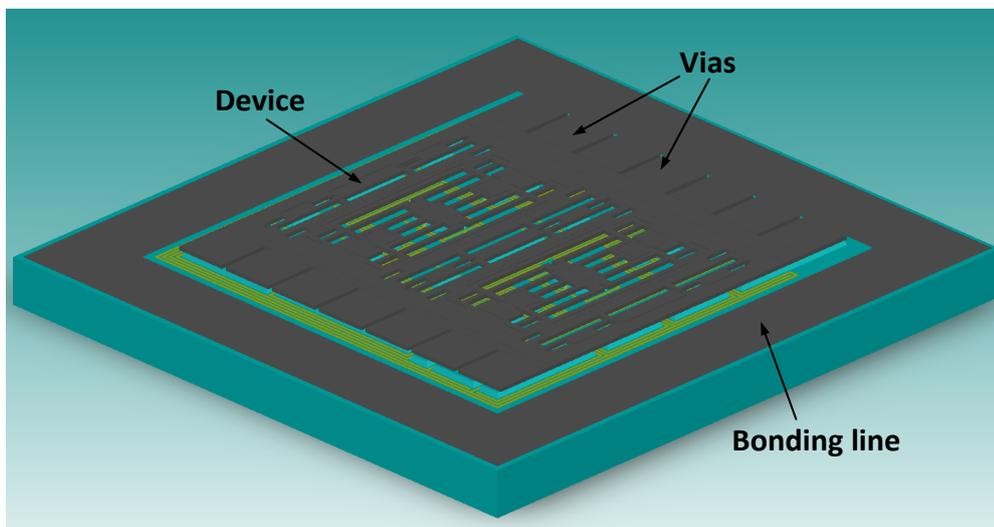
i) Removal of the handle silicon and buried oxide of SOI wafer
