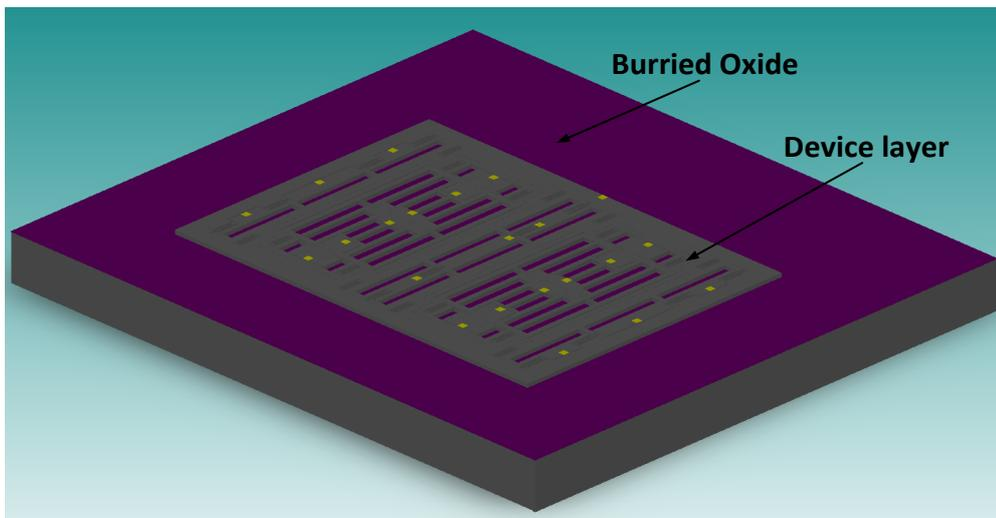
k) Etching of SOI device layer until reaching to the buried oxide layer
