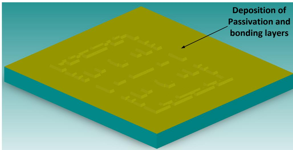
e) Deposition of  $\text{Si}_3\text{N}_4$  passivation layer and Cr/Au bonding line
