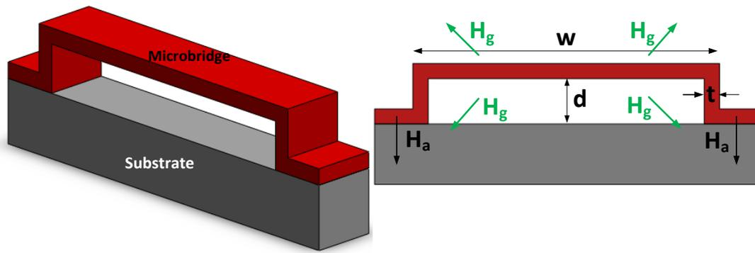
Figure 2.9: Microbridge structure of pirani gauge.
