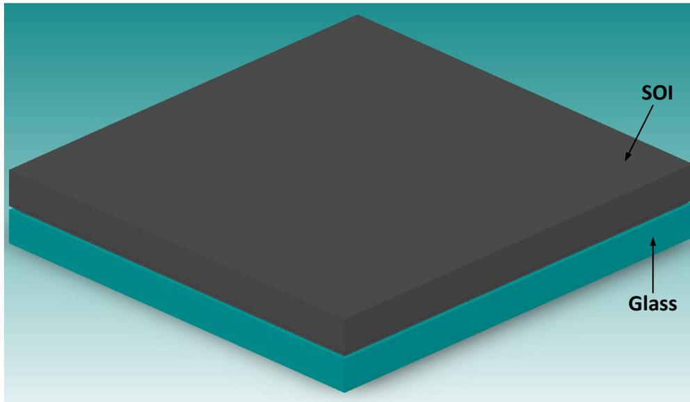
h) Anodic bonding of glass and SOI wafers
