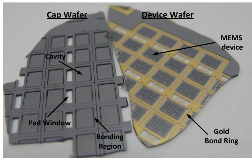
Figure 4.8: The device wafer can easily be separated from the silicon cap wafer, showing that wafer level vacuum packaging is unsuccessful.
