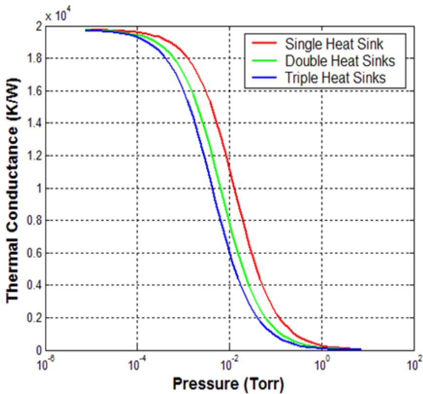
Figure 2.14: The effect of heat sinks on the pirani gauge performance.
