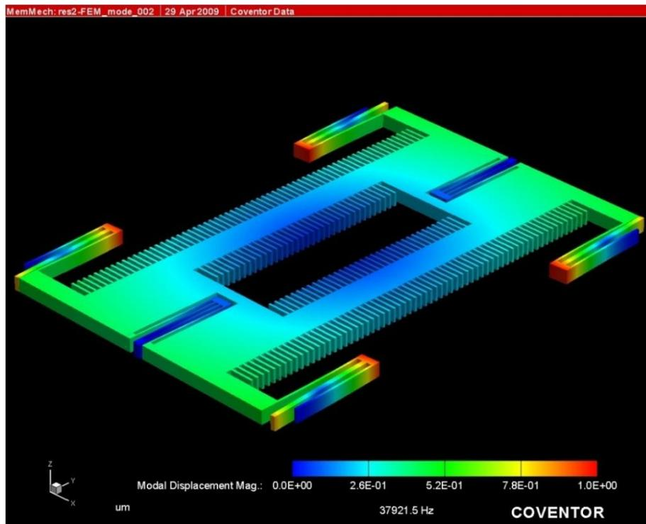
Figure 2.5: Undesired mode which has a movement to out of plane (second mode) at 37.9 kHz.
