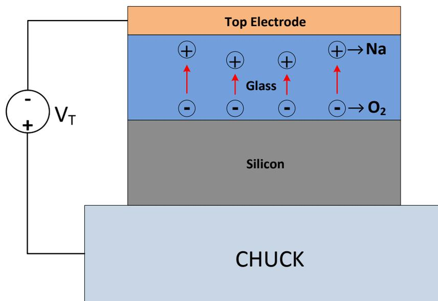
Figure 1.10: A basic anodic bonding scheme.
