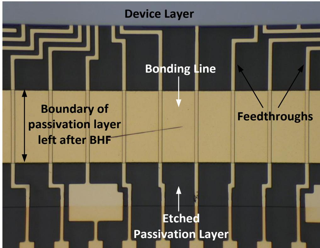
Figure 3.16: The optical microscope view of a gyroscope die released by BHF.
