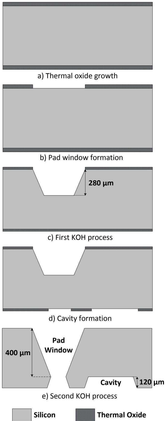
Figure 3.24: The main process steps for the cap wafer fabrication.
