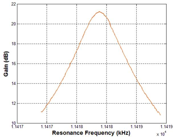
Figure 4.4: Measured resonance characteristic of the resonator Design-1 at 1.8mTorr.
