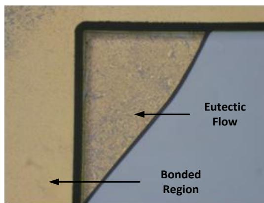
Figure 3.7: An optical microscope picture from bond#6. Higher bond forces resulted in eutectic flow on device area.
