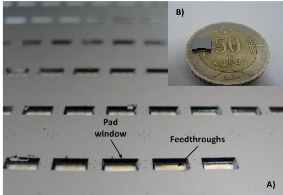
Figure 3.26: The view of device wafer with lateral feedthroughs after wafer level vacuum packaging: (a) top view, (b) view of a gyroscope die after dicing.
