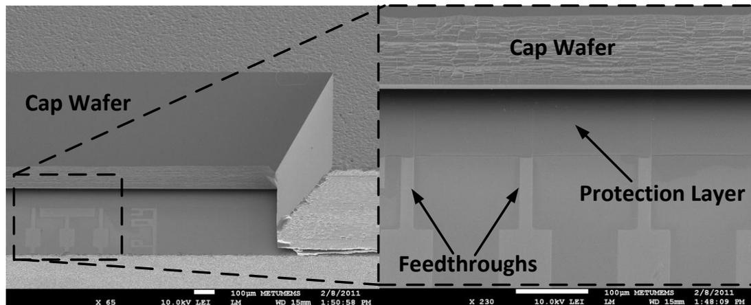
Figure 3.27: SEM pictures of a die from SNW#9 vacuum packaged by glass frit bonding.
