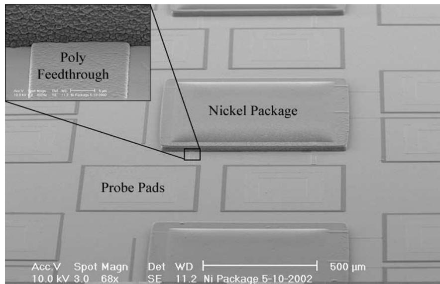
Figure 1.7: A SEM picture of Nickel thin film package developed in 2004 [16].
