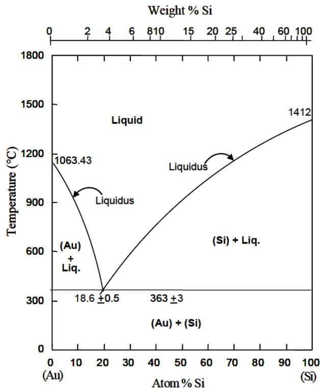
Figure 3.1: The phase diagram of Au-Si eutectic system [53].
