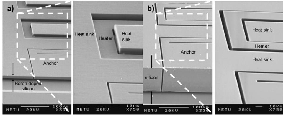
Figure 2.16: The previously developed pirani gauges at METU: (a) DWP pirani gauge, (b) SOG pirani gauge [48].
