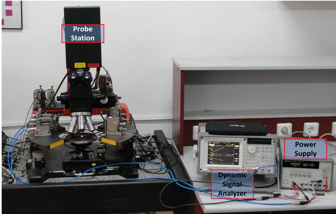
Figure 4.1: The functionality test setup for gyroscopes and resonators.
