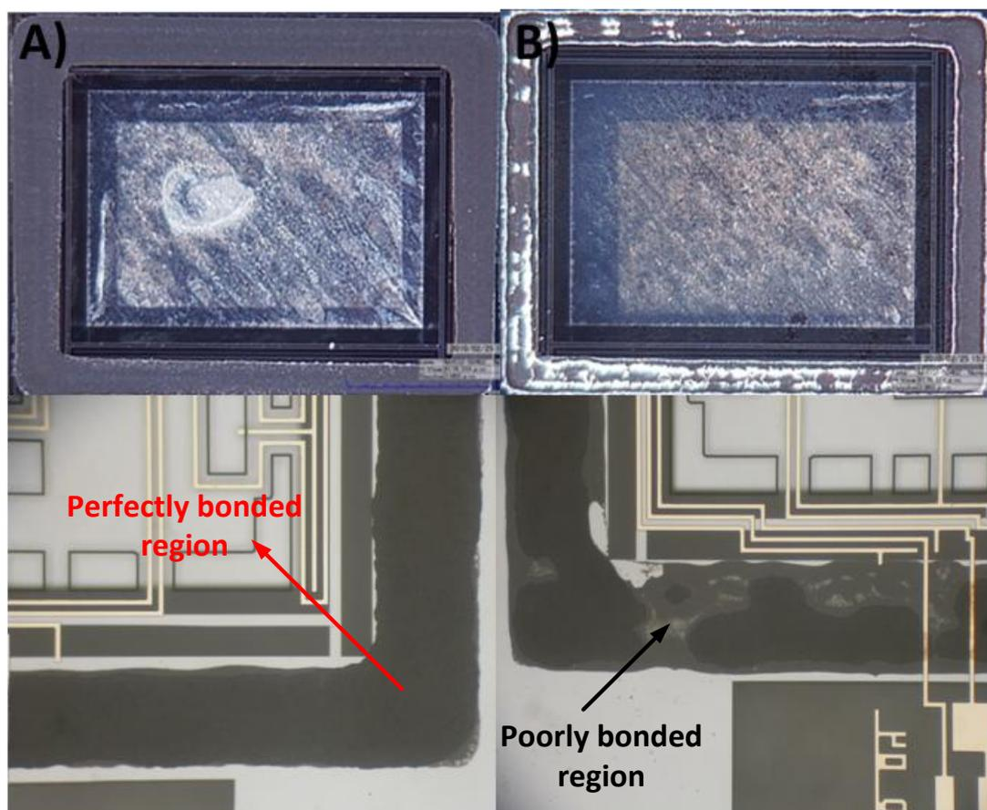
Figure 3.11: The evaluation of bond quality by optical microscope: (a) successful bonding, (b) unsuccessful bonding.
