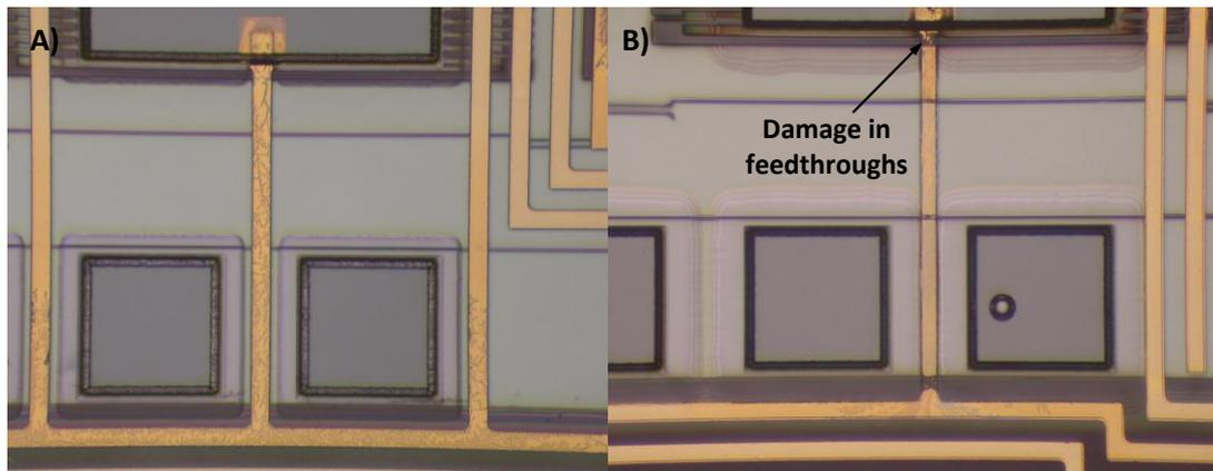
Figure 3.28: Two packaged dies at a temperature of 420°C: (a) longer cooling, (b) shorter cooling.
