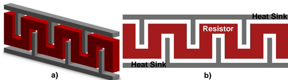
Figure 2.17: The meander shaped suspended microbridge resistor with dual heat sinks structure used in this study: (a) isometric view, (b) top view.
