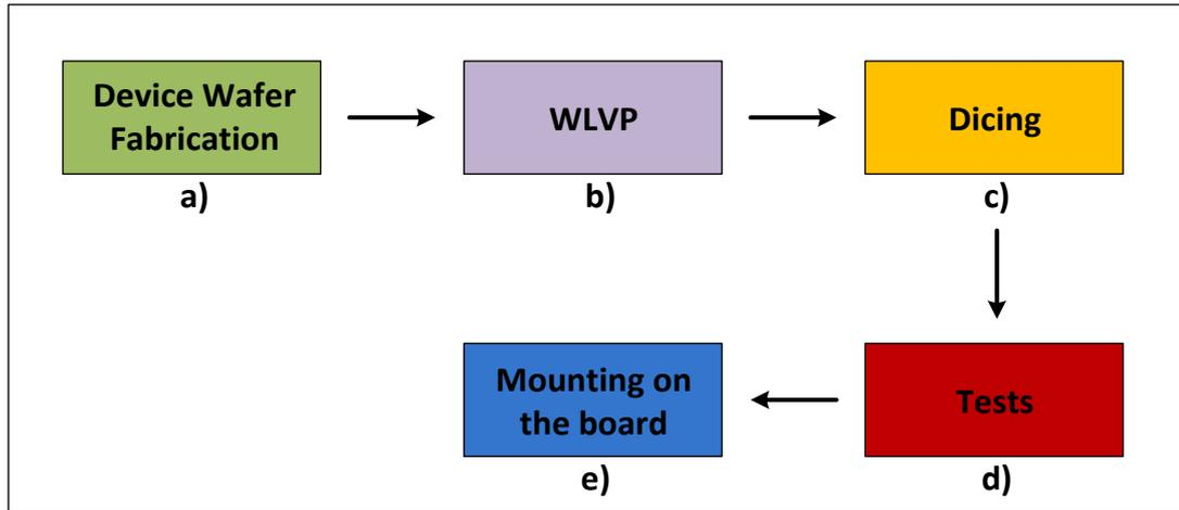
Figure 1.4: The basic concept of wafer level vacuum packaging: (a) fabrication of device wafer, (b) wafer level vacuum packaging process using one of selected wafer level vacuum packaging techniques, (c) dicing of the packaged device wafer to obtain individual dies, (d) tests, (e) mounting the vacuum packaged functional dies on the board for final tests.
