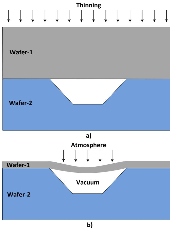
Figure 3.4: The principle of deflection test used for the evaluation of the bond quality: (a) before thinning, (b) after thinning.
