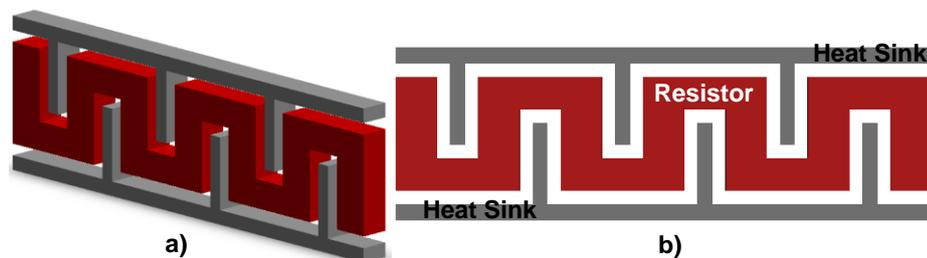
Figure 2.17: The meander shaped suspended microbridge resistor with dual heat sinks structure used in this study: (a) isometric view, (b) top view.
