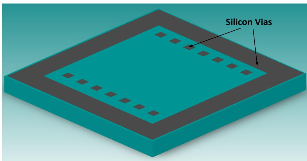
a) Pyrex glass wafer with highly doped silicon vias
