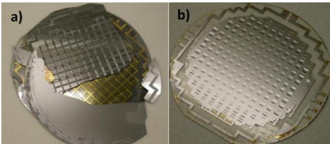
Figure 3.8: The view of bonded wafer pairs after the bond quality test: (a) bond#1. The cap easily separated from the device wafer, (b) bond#5. The cavities are deflected to downwards, which proves the vacuum.
