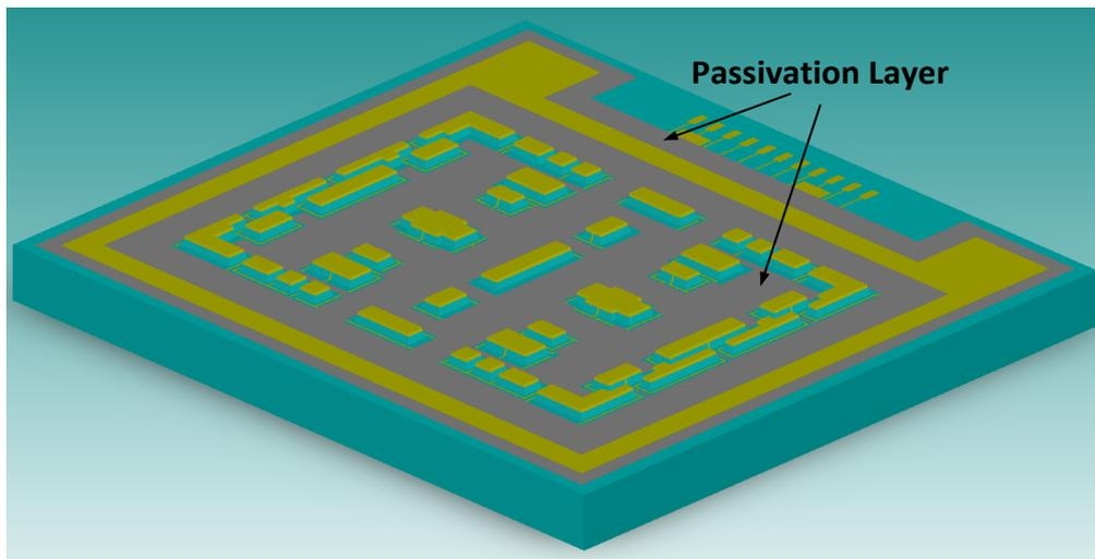
g) Formation of  $\text{Si}_3\text{N}_4$  passivation layer
