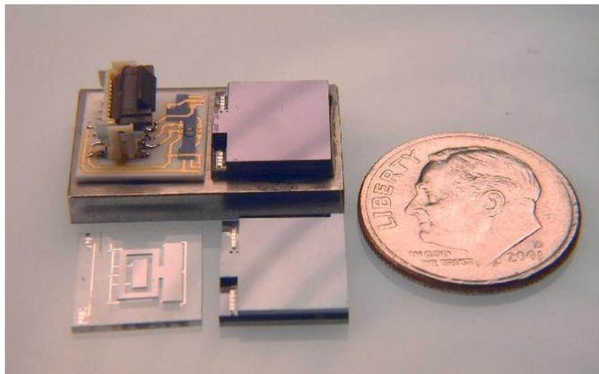
Figure 3.9: Chip level packages developed in [62].
