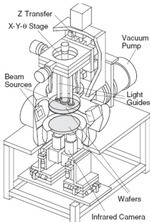
Figure 1.11: Special bonding equipment for surface plasma activated bonding [26].
