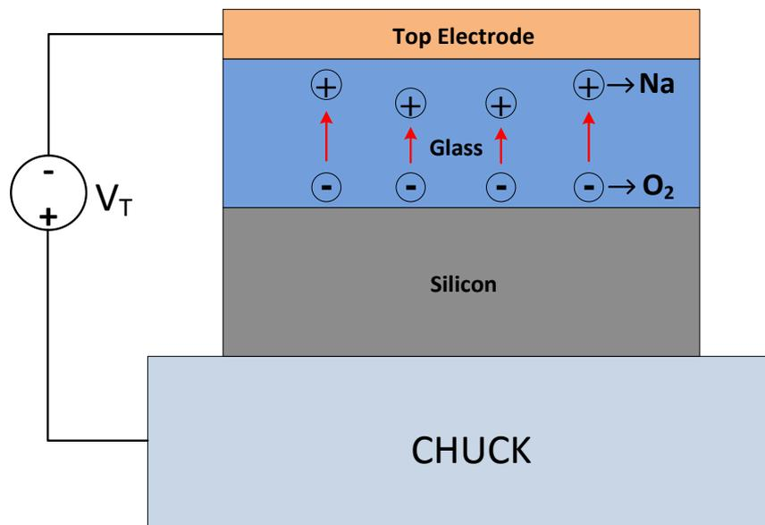
Figure 1.10: A basic anodic bonding scheme.
