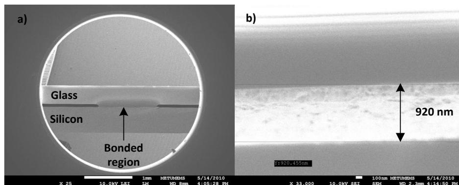
Figure 3.6: SEM pictures of bond#4: (a) the cross sectional view of eutectically bonded glass-silicon wafers, (b) the view of bonding interface.
