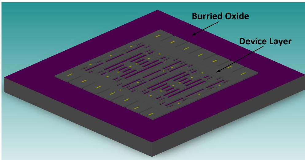
g) Etching of SOI device layer until reaching to the buried oxide layer
