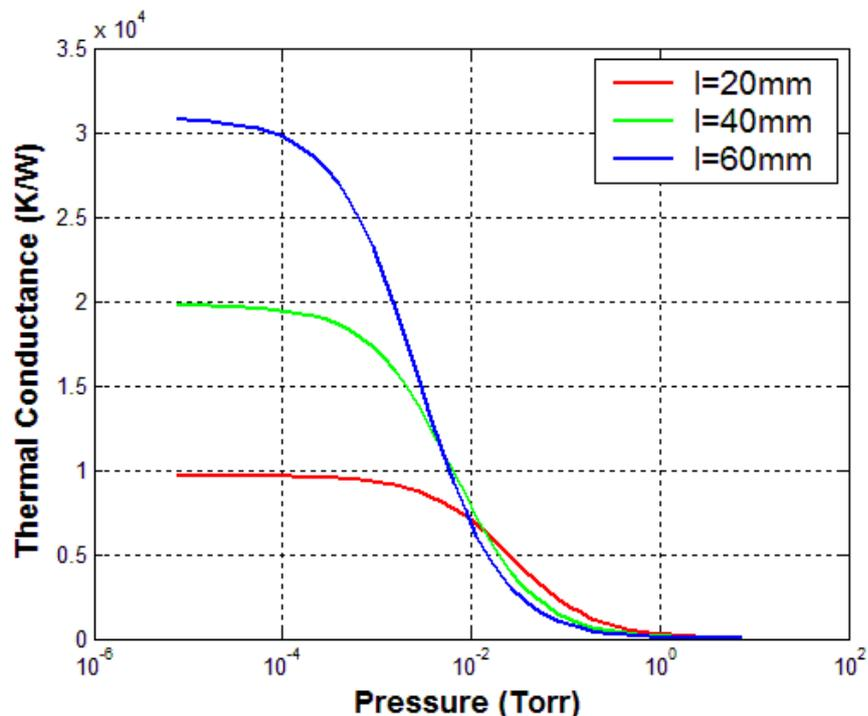
Figure 2.10: The effect of resistor length on the performance of a pirani gauge.
