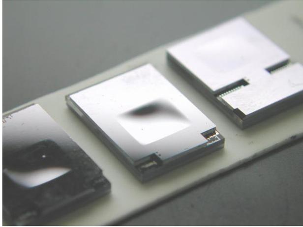
Figure 3.10: Packages subjected to the deflection test for the evaluation of vacuum quality [34].
