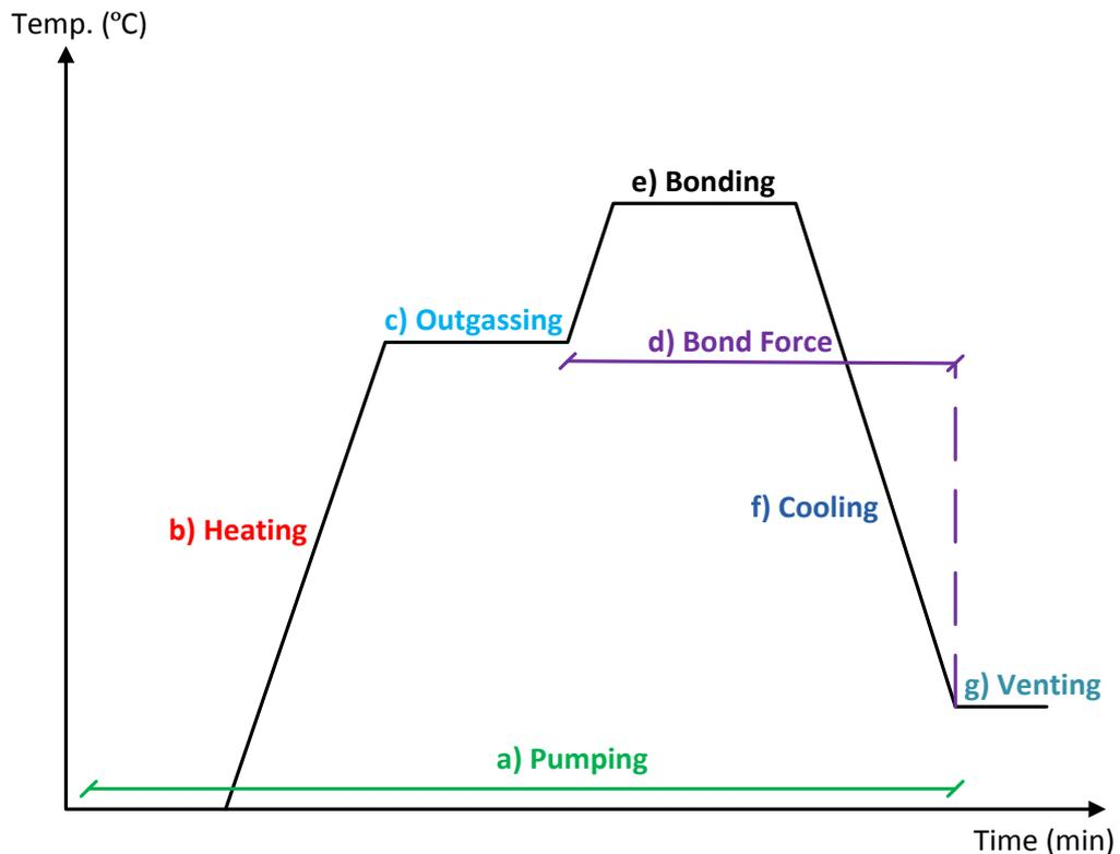
Figure 3.3: The generic bond recipe for Au-Si eutectic bonding.
