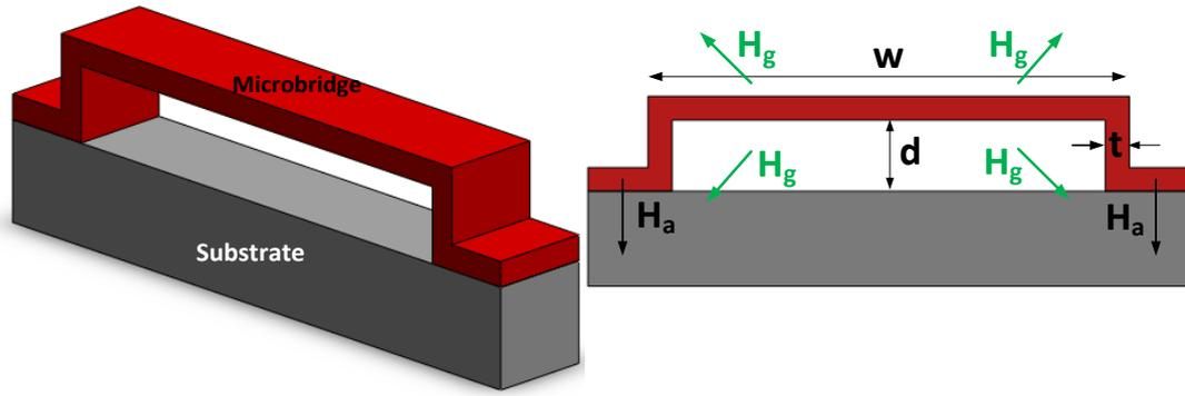
Figure 2.9: Microbridge structure of pirani gauge.
