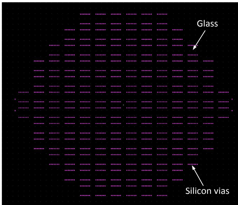
Figure 3.21: The initial layout for the fabrication of glass wafer with highly doped silicon vias.
