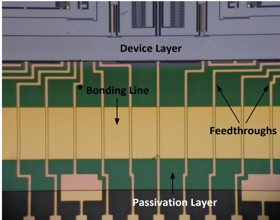
Figure 3.17: The optical microscope view of a gyroscope die released by RIE.
