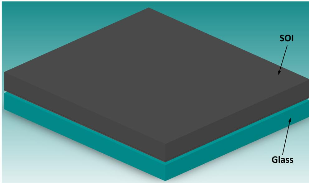
1) Anodic bonding of glass and SOI wafers
