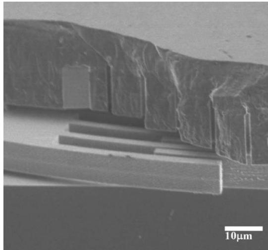
Figure 1.8: Cross section view of sealed resonator die by thin film packaging [20].
