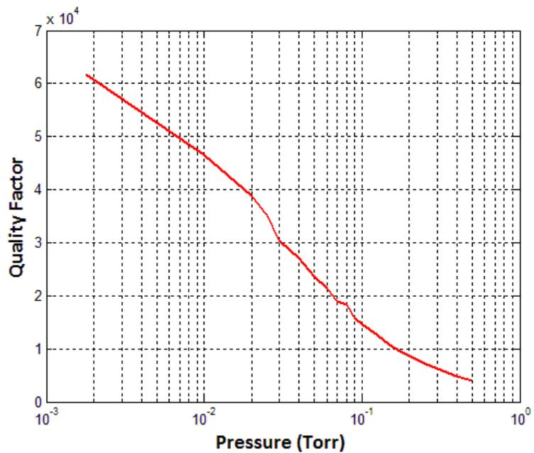
Figure 4.5: The quality factor versus ambient pressure for a resonator die.
