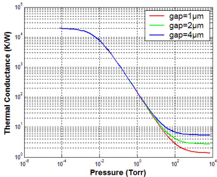
Figure 2.13: The effect of gap between the resistor and heat sinks on the performance of a pirani gauge.
