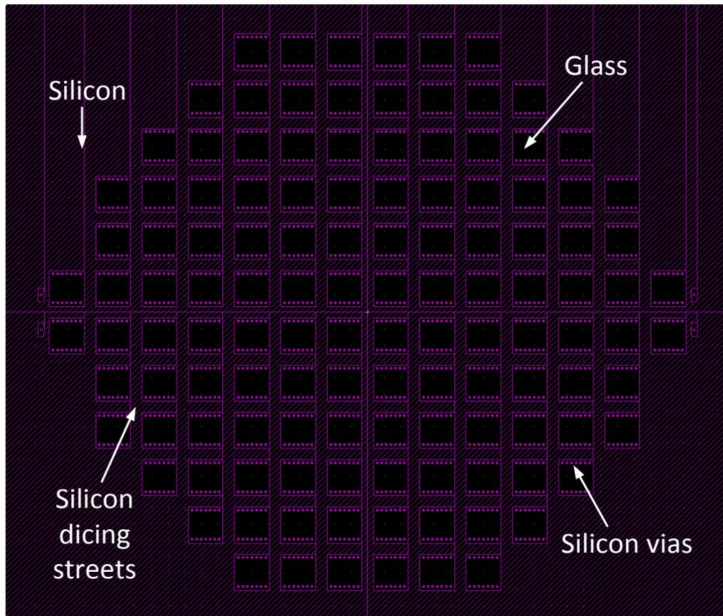
Figure 3.23: The modified layout for the fabrication of glass wafers with highly doped silicon vias.
