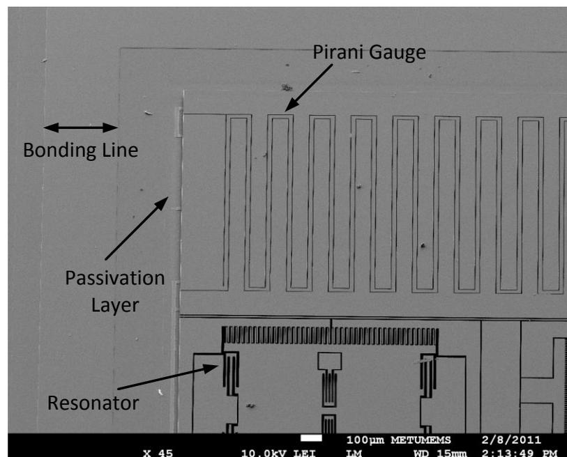
Figure 3.18 : SEM photo of fabricated pirani gauge and resonator.
