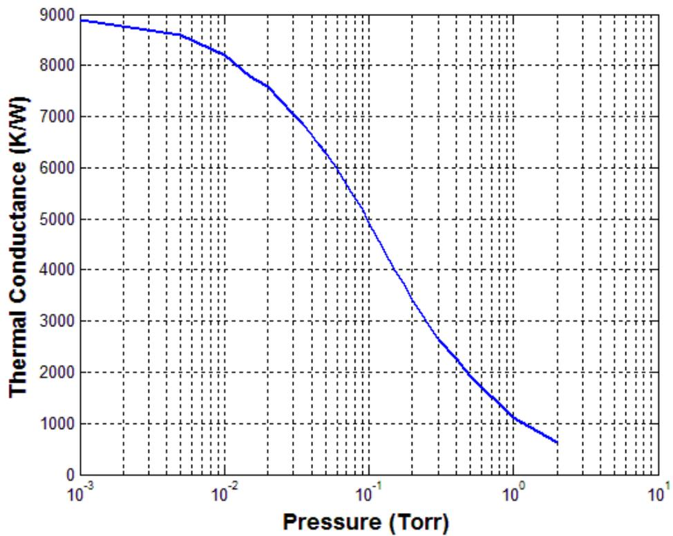
Figure 4.7: The vacuum response of the pirani gauge Design-2.
