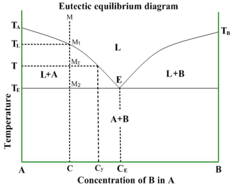
Figure 1.12: A basic eutectic phase diagram.
