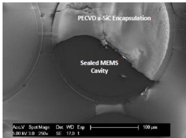
Figure 1.9: Top view of a die sealed by deposition of PECVD a-Si [21].
