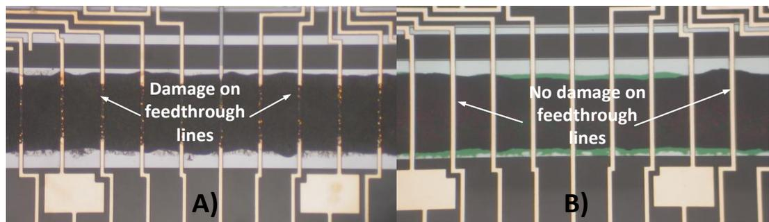
Figure 3.13: The view of gold feedthroughs after glass frit bonding at 435C for a holding period of 60 min: (a) bonding directly on the gold feedthroughs, (b) bonding when silicon nitride protection layer is used between the gold feedthroughs and glass frit.
