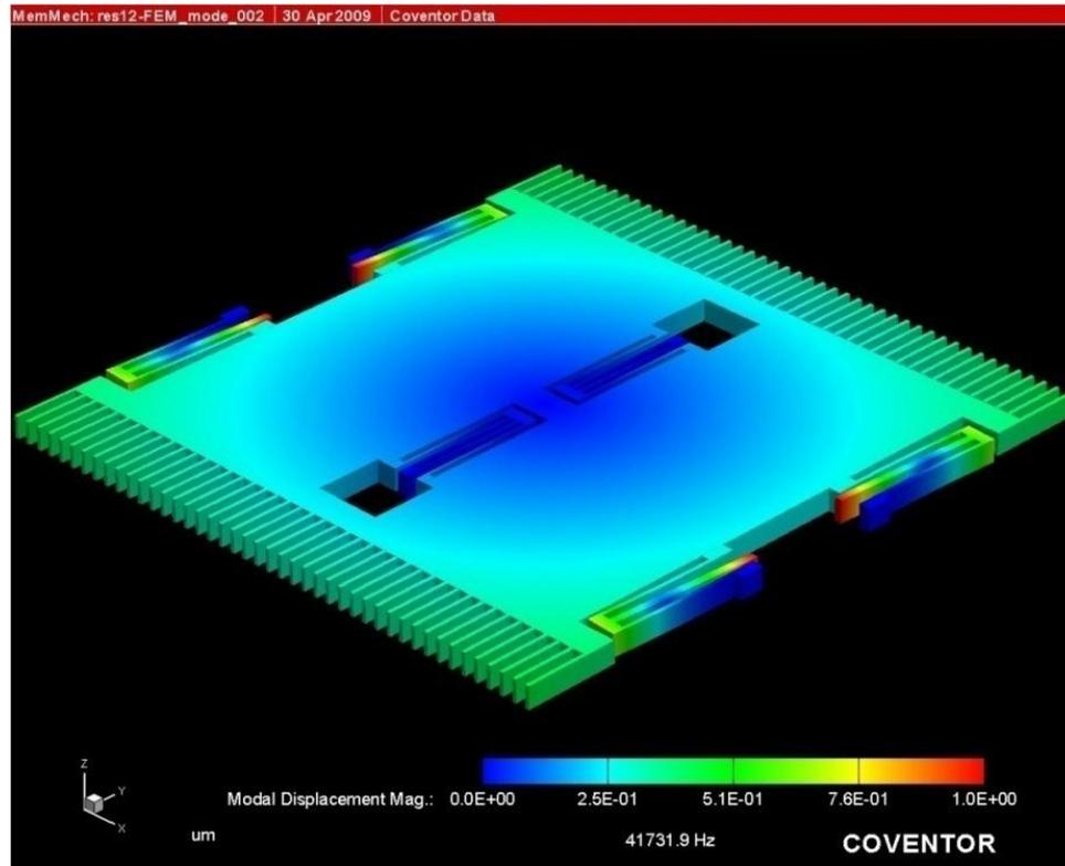
Figure 2.7: Undesired mode which has a movement to out of plane (second mode) at 41.7 kHz.
