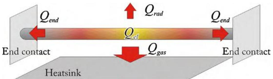
Figure 2.8: Heat loss mechanisms in pirani gauge [51].
