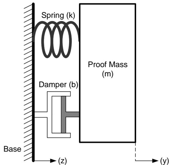
Figure 2.1: A simple micromachined resonator device [40].
