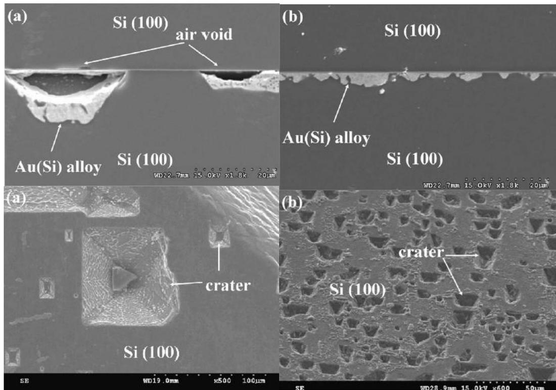
Figure 3.2: The SEM images of bonded wafers: (a) Au/crystal Si eutectic bonds. (b) Au/amorphous Si eutectic bonds [58].
