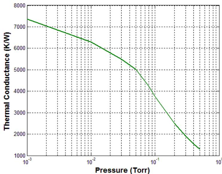
Figure 4.6: The vacuum response of the pirani gauge Design-1.
