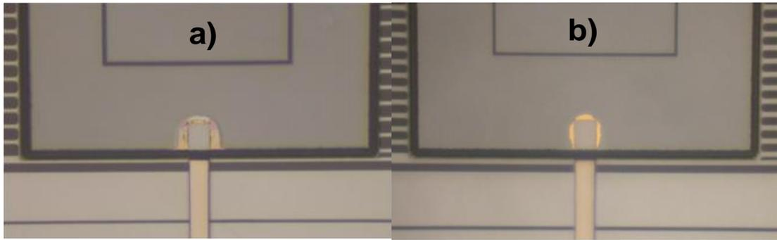
Figure 3.19: The view of contact regions after the release process: (a) photograph of a die released by BHF, (b) photograph of a die released by RIE.
