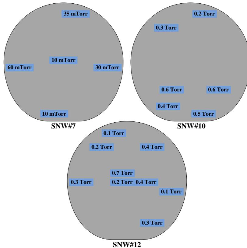
Figure 4.10: The measured pressure distribution over the sensor wafers 7, 10, and 12 that are wafer level vacuum packaged using glass frit bonding.
