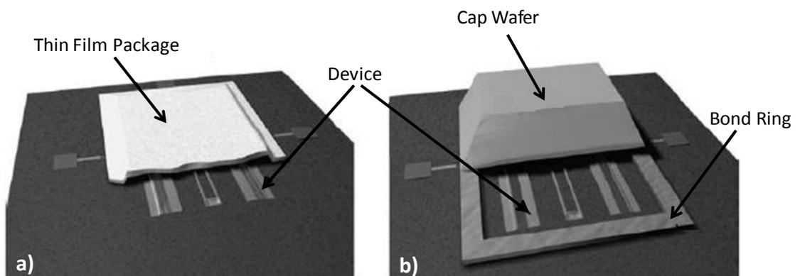
Figure 1.5: Two basic wafer level vacuum packaging approaches: (a) packaging using thin film deposition, (b) packaging using wafer bonding [16].
