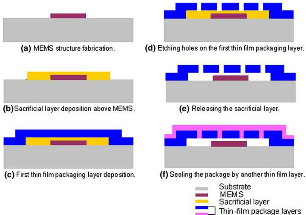
Figure 1.6: A conceptual process flow for thin film packaging [19].
