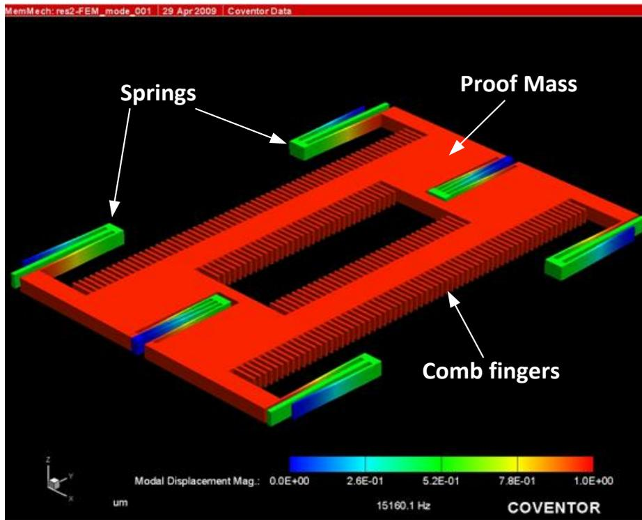
Figure 2.4: First mode of Design-1. The frequency is 15.1 kHz, which is close to the designed frequency of 15 kHz.
