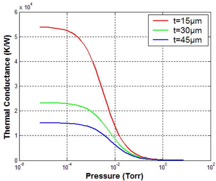
Figure 2.12: The effect of resistor thickness on the performance of a pirani gauge.
