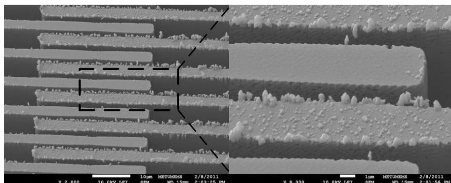
Figure 4.9: The polymer residues detected over the finger regions.
