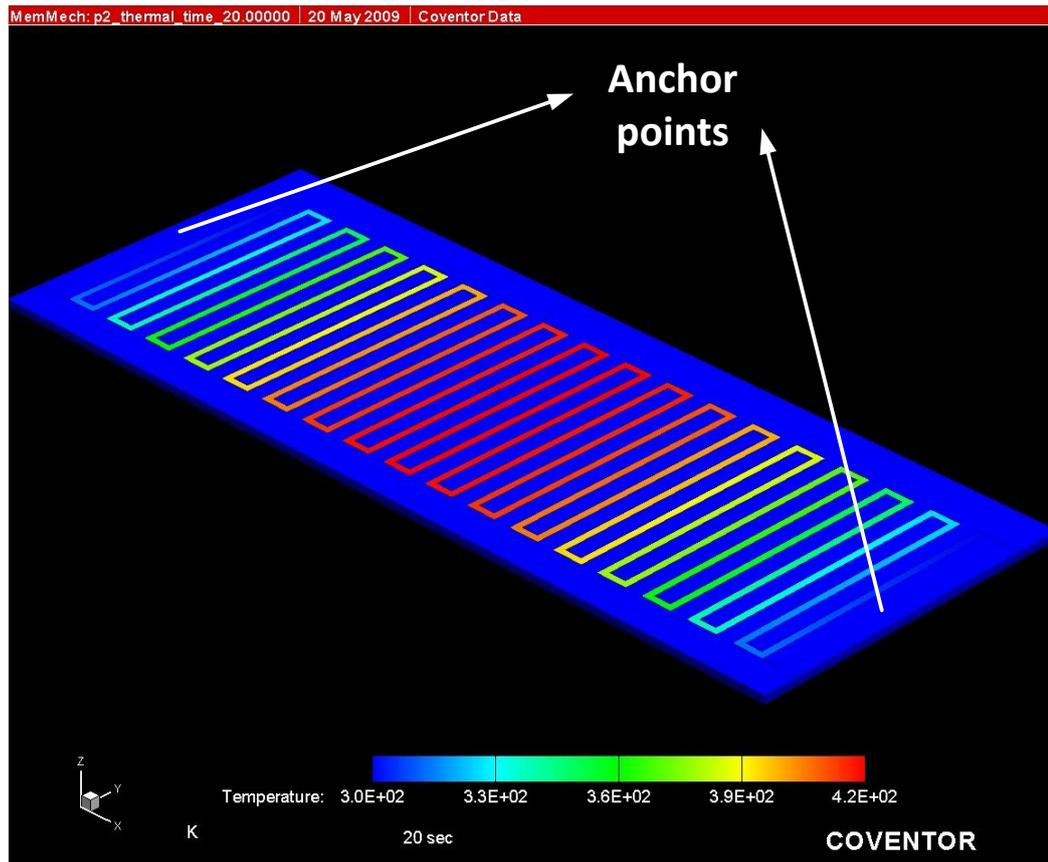
Figure 2.15: The temperature distribution on the resistor.
