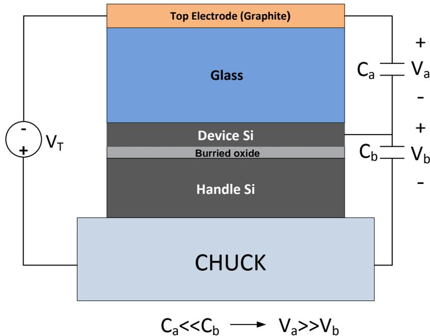
Figure 3.14: The view of anodic bonding scheme.
