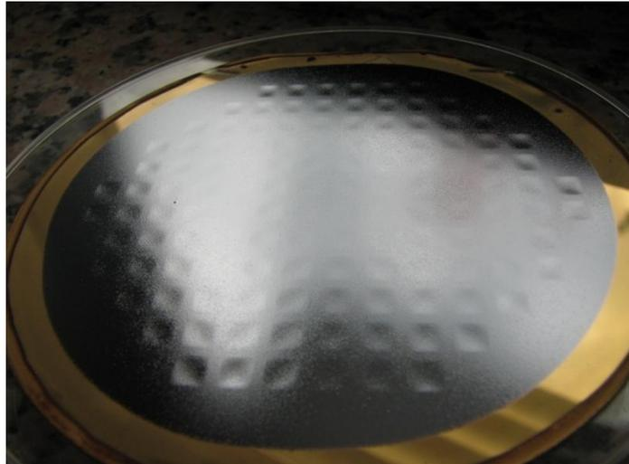
Figure 3.5: The view of bond#4 after the deflection test. The thinned silicon layers deflected to downwards due to the vacuum inside the cavities.
