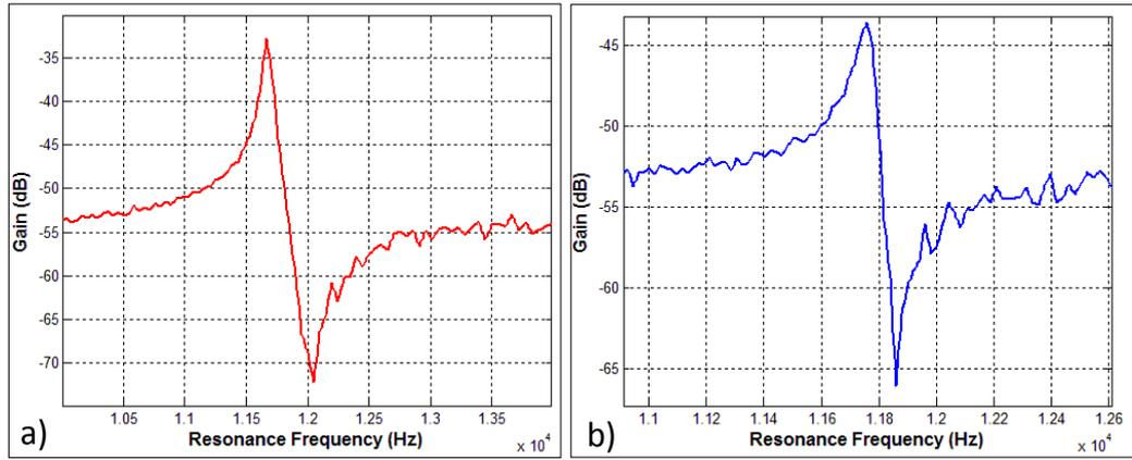
Figure 4.2: Measured resonance characteristics at atmosphere: (a) gyroscope, (b) resonator.
