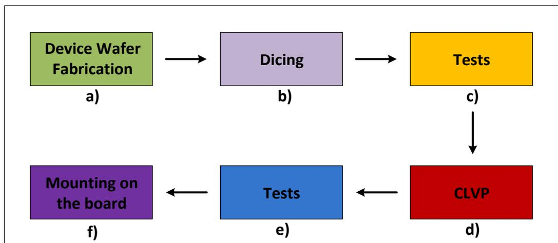
Figure 1.3: The basic concept of die level vacuum packaging: (a) fabrication of device wafer, (b) dicing of the device wafer to obtain individual dies, (c) functionality tests, (d) die level packaging of dies one by one, (e) tests of vacuum packaged dies to see whether vacuum packaging process is successful or not, (f) mounting the vacuum packaged dies on the board for final tests.
