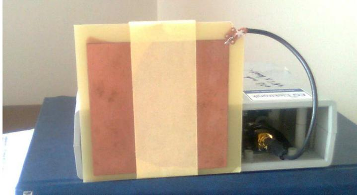
Figure 7.20 Active RFID reader and patch antenna used in the experimental work
