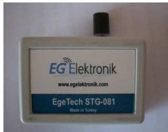
Figure 7.19 Active RFID tag with JJB antenna attached
